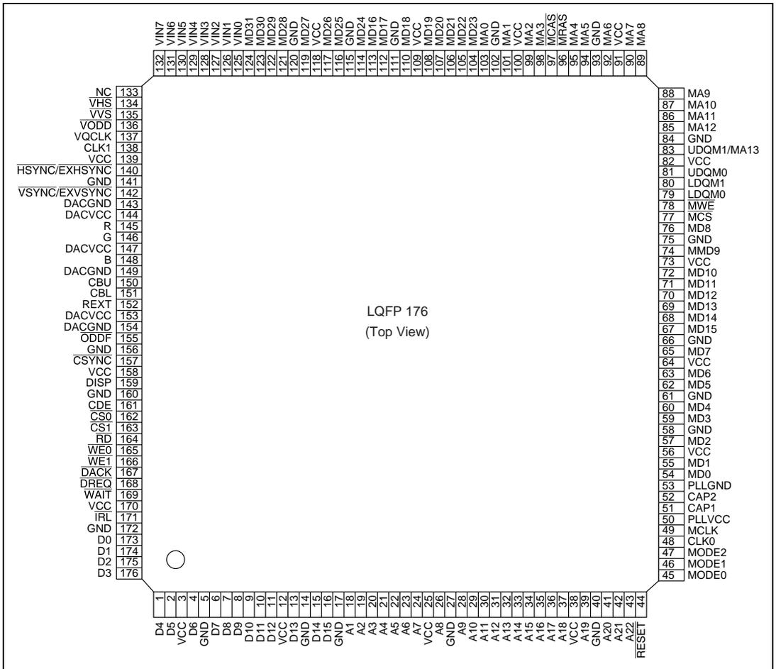
**Figure 2.2 Pin Arrangement**
