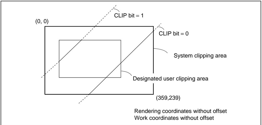
**Figure 3.45 Example of Clipping Specification**
