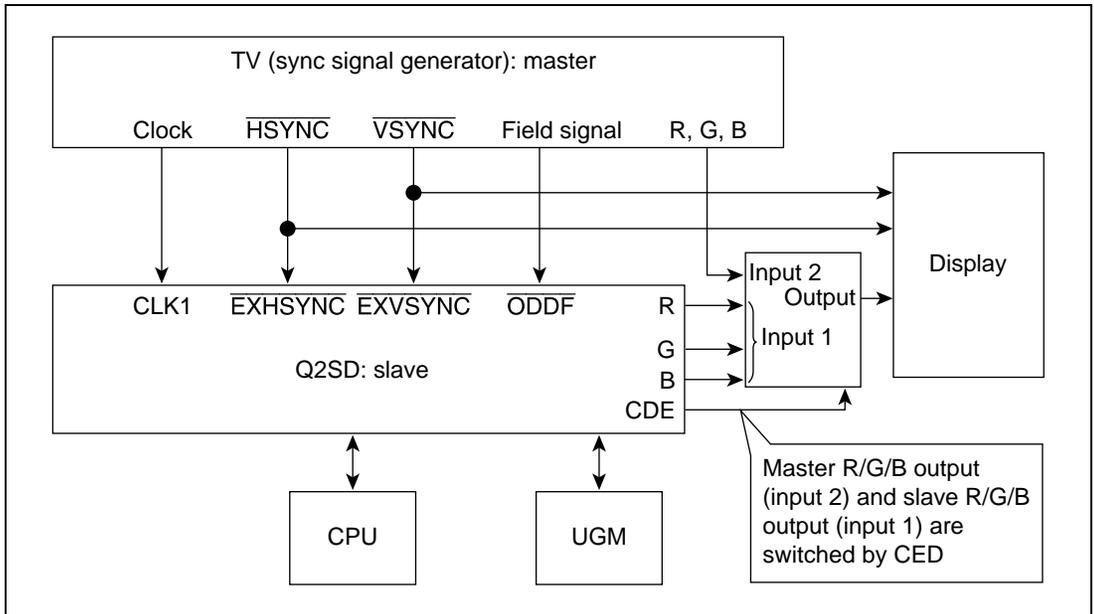
**Figure 3.35 Signal Flow in TV Sync Mode**
