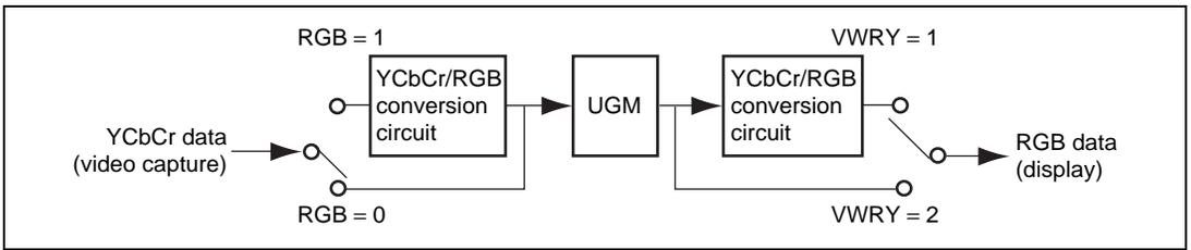
**Figure 3.67 Conversion of YCbCr Data into RGB Format**
