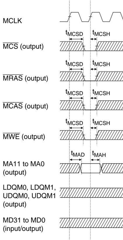
**Figure 7.11 (2) UGM Mode Register Setting Cycle Timing**
