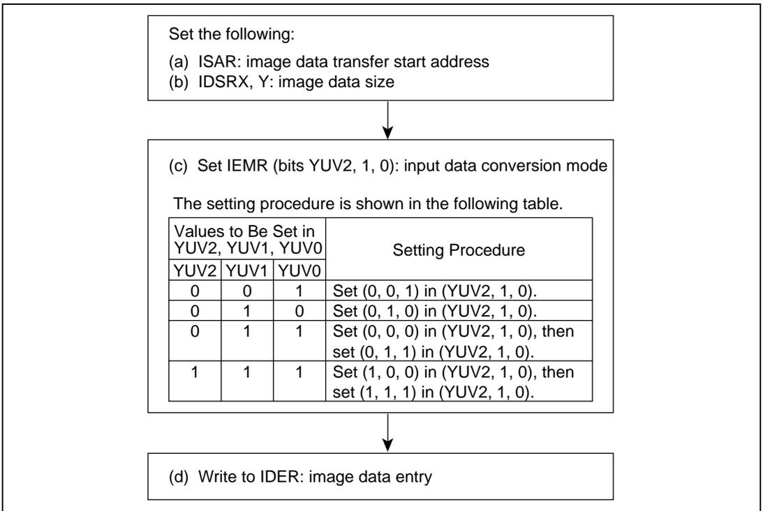
**Figure 3.5 Register Setting Procedure for  $\Delta$ YUV/YUV-to-RGB Conversion**
