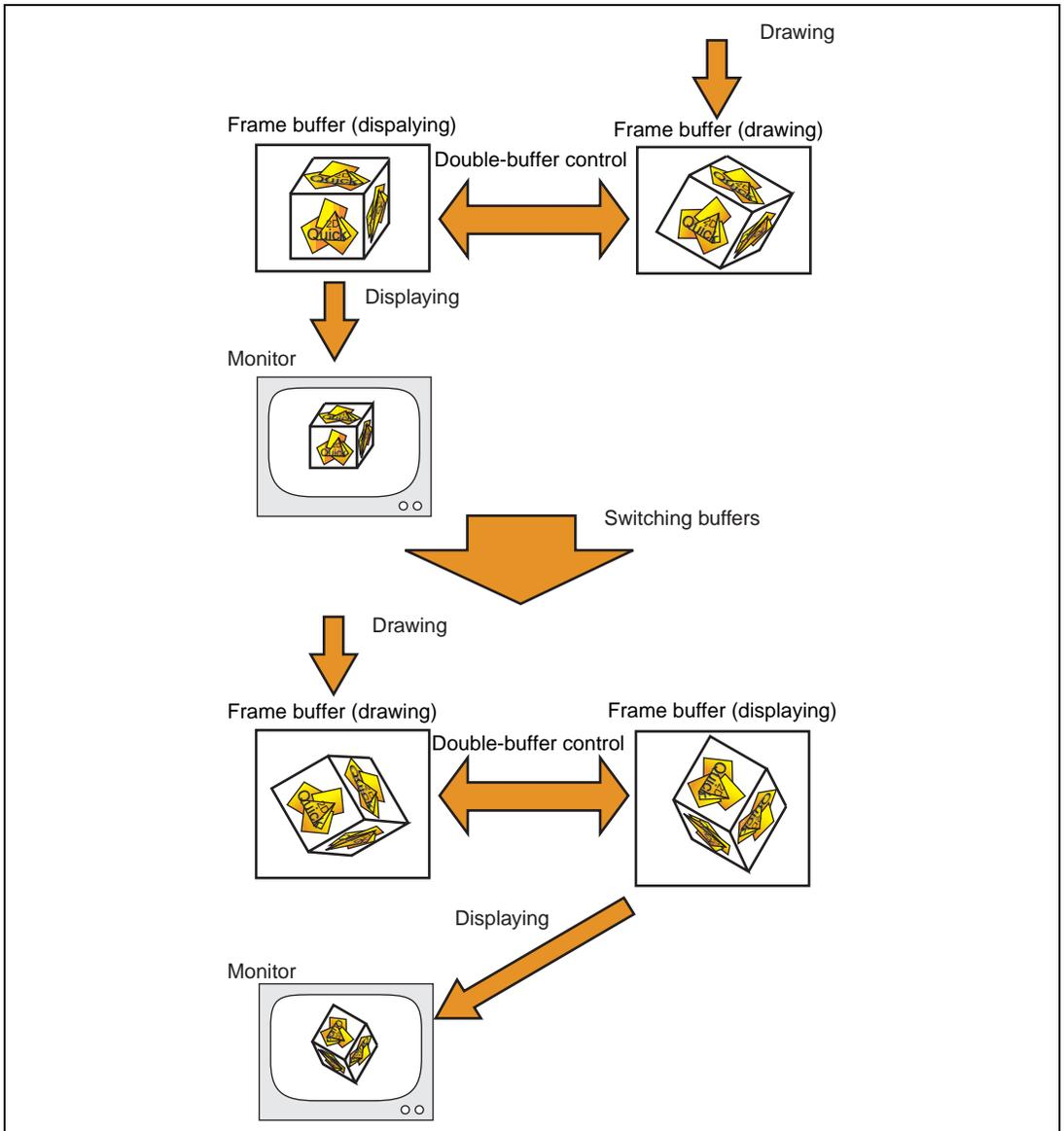
Figure 1.4 Double-Buffering Architecture
