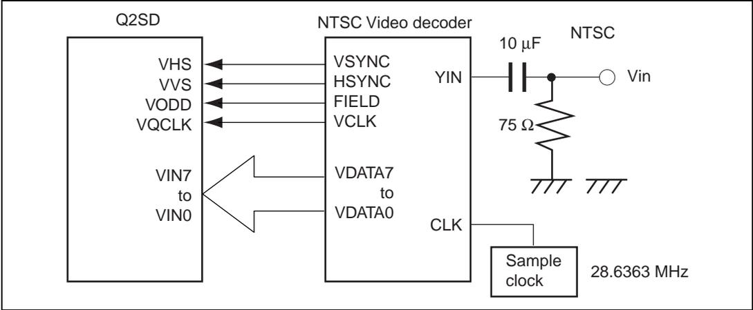
**Figure 2.6 Example of Connection of Video Input Pins**
