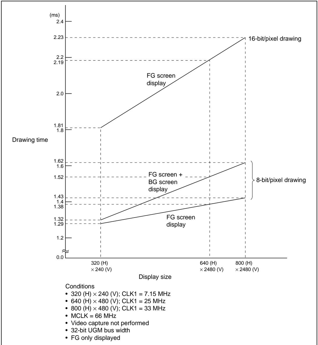
**Figure I.1 POLYGON4C Drawing Performance when FST = 0**
