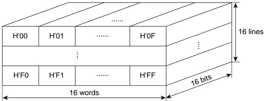
**Figure 3.7 Configuration of One Memory Unit (512 Bytes)**
