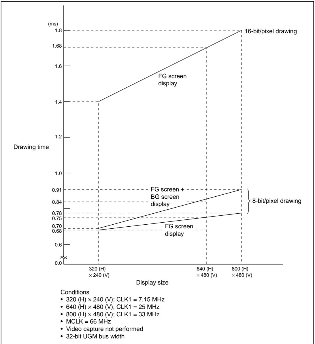
**Figure I.2 POLYGON4C Drawing Performance when FST = 1
