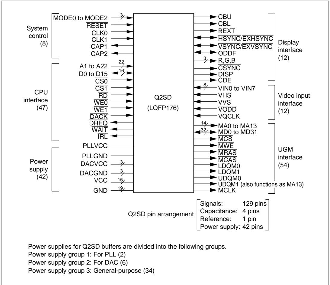
**Figure 2.1 Pin Configuration**
