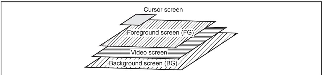
**Figure 3.26 Configuration of the Display Screen for Q2SD**
