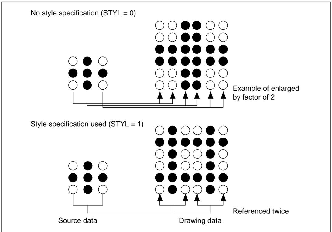
**Figure 3.44 Example of Source Style Specification**
