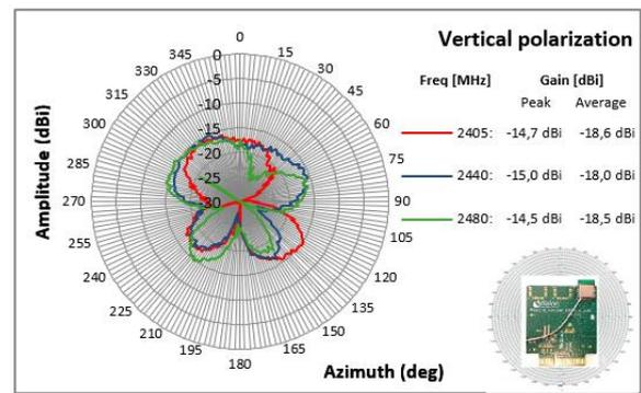
Figure 21. Radiation pattern for YZ-plane, vertical polarization
