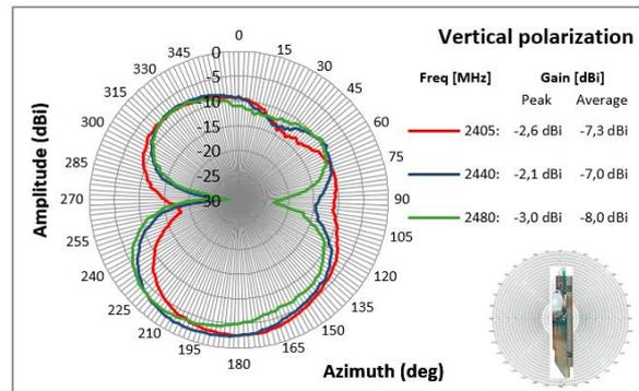
Figure 19. Radiation pattern for XZ-plane, vertical polarization
