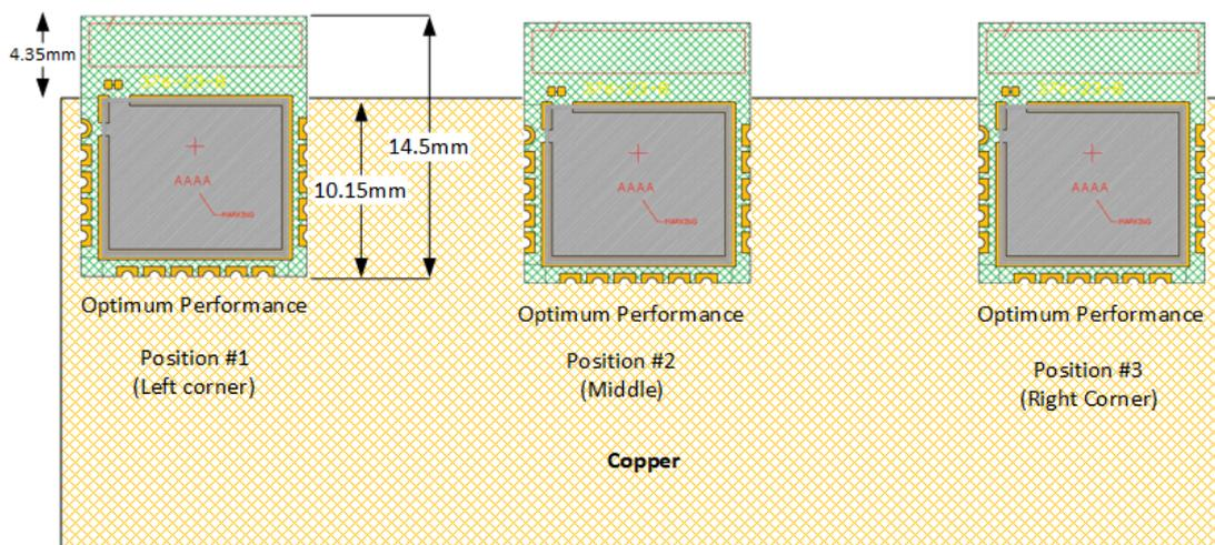
Figure 9. Installation locations for optimum antenna performance
