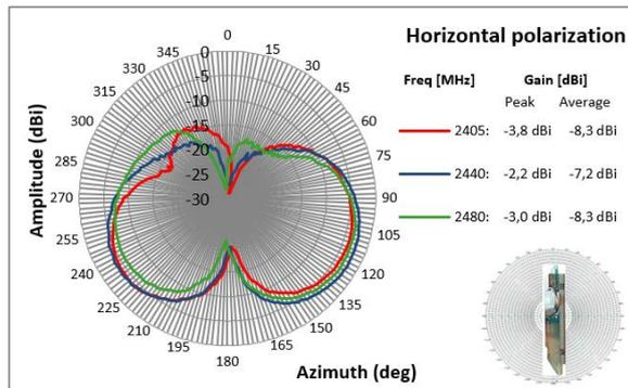
Figure 18. Radiation pattern for XZ-plane, horizontal polarization
