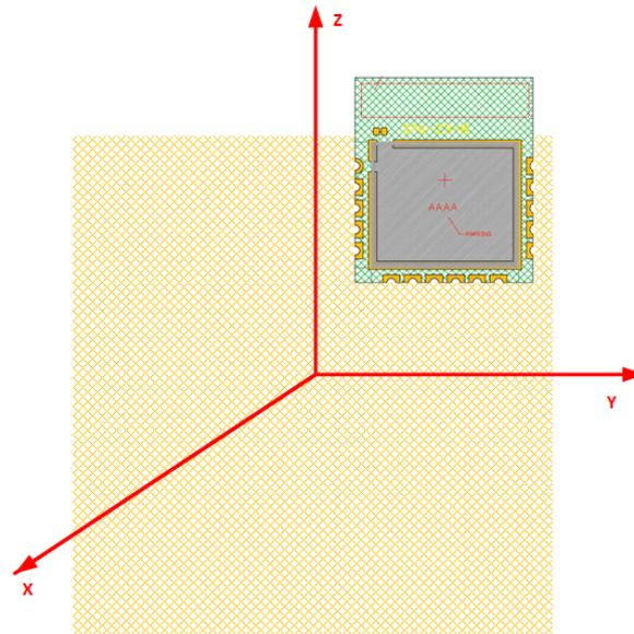
Figure 15. Measurement plane definition
