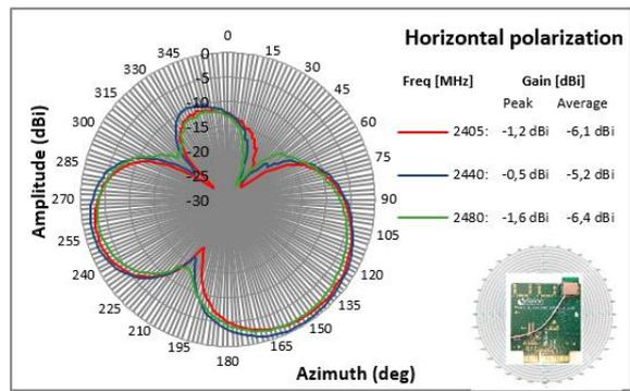
Figure 20. Radiation pattern for YZ-plane, horizontal polarization
