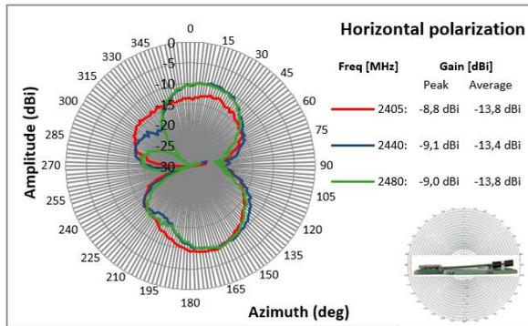
Figure 16. Radiation pattern for XY-plane, horizontal polarization
