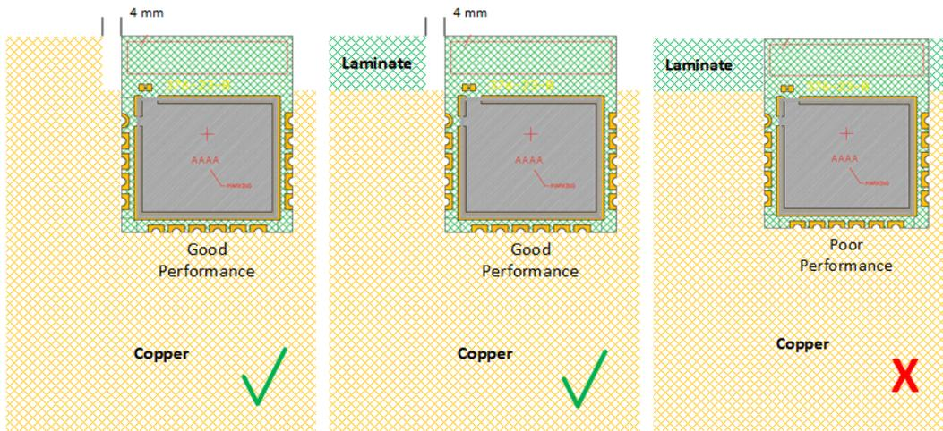
Figure 10. Antenna performance in proximity of copper (left), laminate (middle), and laminate under antenna (right) The actual TINY™ module evaluation board layout that has been used to conduct measurements is shown in Figure 11.
