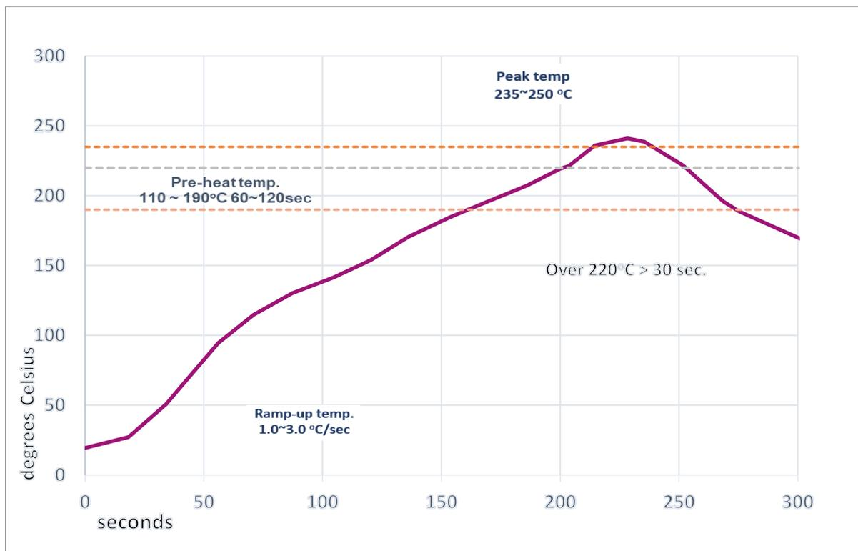
Figure 22. Recommended reflow profile for lead free solder
