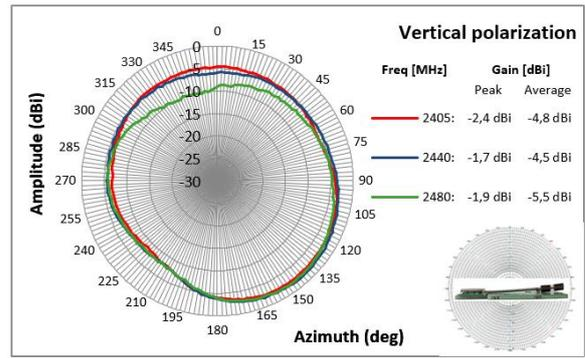
Figure 17. Radiation pattern for XY-plane, vertical polarization
