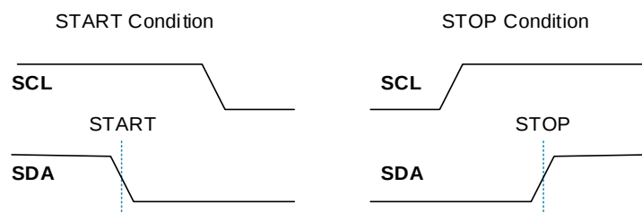
Figure 5. START and STOP Condition Waveform
