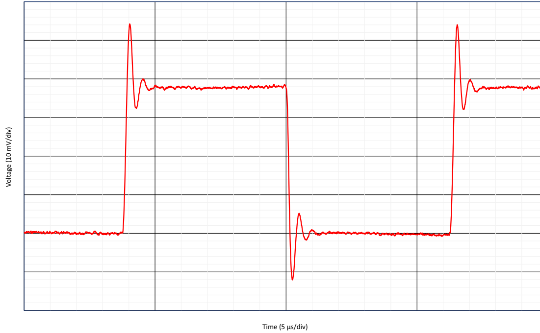
Figure 114: Small Signal Non-Inverting Step Response G = -1 \text{ V/V} , R_L = 50 \text{ k}\Omega , C_L = 60 \text{ pF} , \text{BW} = 2 \text{ MHz}
