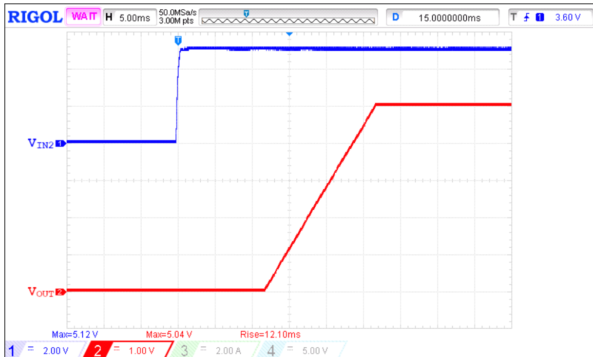
Figure 4. Typical Turn ON operation waveform for V_{IN2} = 5\text{ V} , C_{SS} = 220\text{ nF} , R_{LOAD} = 100\text{ }\Omega , C_{LOAD} = 2\text{ }\mu\text{F}
