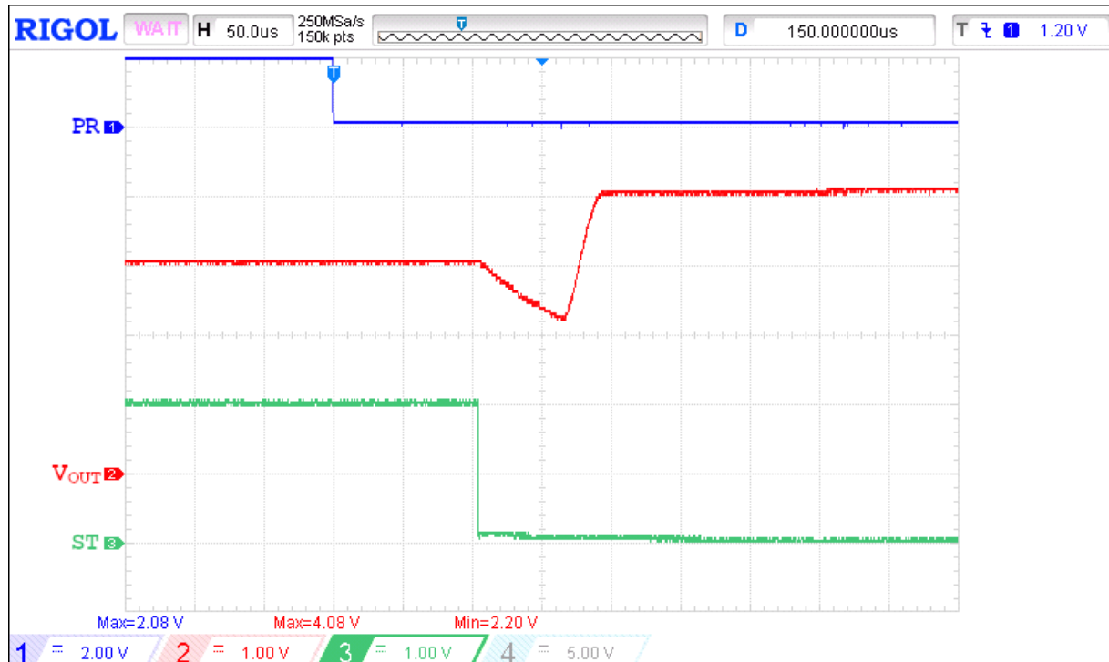
Figure 10. Switchover operation waveform for V_{IN1} = 3\text{ V} , V_{IN2} = 4\text{ V} , C_{SS} = 220\text{ nF} , SEL = 0\text{ V} , PR = \text{High} \rightarrow \text{Low} , R_{LOAD} = 100\text{ }\Omega , C_{LOAD} = 2\text{ }\mu\text{F}
