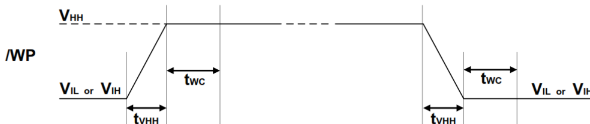
Figure 66. ACC Program Acceleration Timing and Voltage Levels
