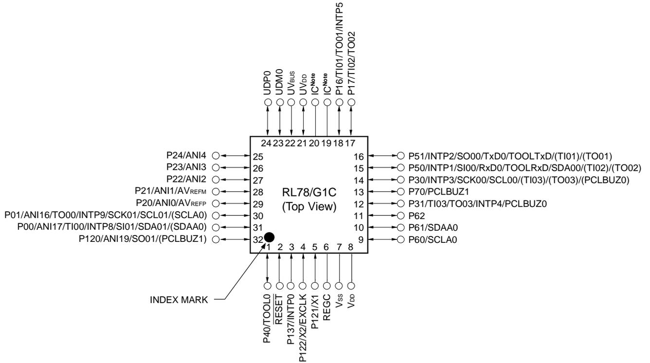
**Note** IC: Internal Connection Pin Leave open.
