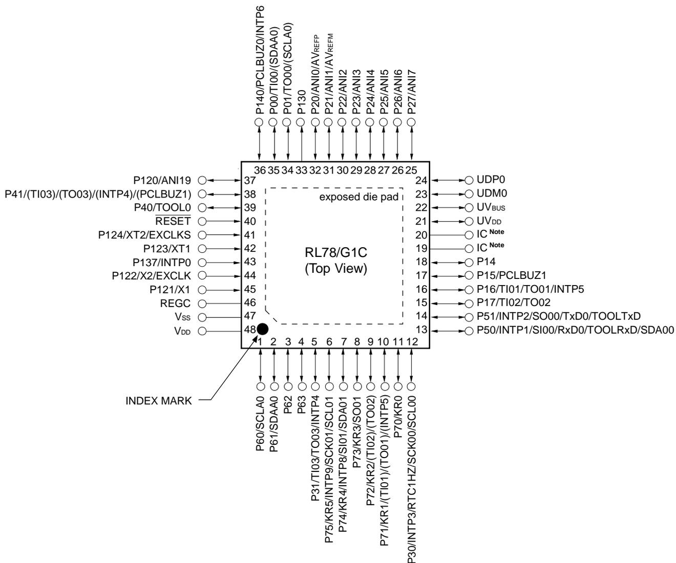
**Note** IC: Internal Connection Pin Leave open.
