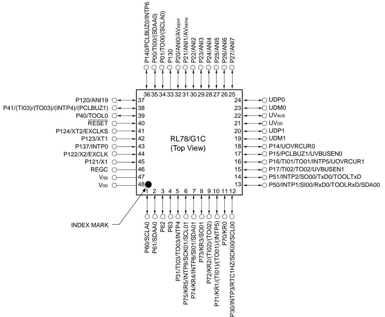
**Caution** Connect the REGC pin to V<sub>SS</sub> via a capacitor (0.47 to 1 μF).
