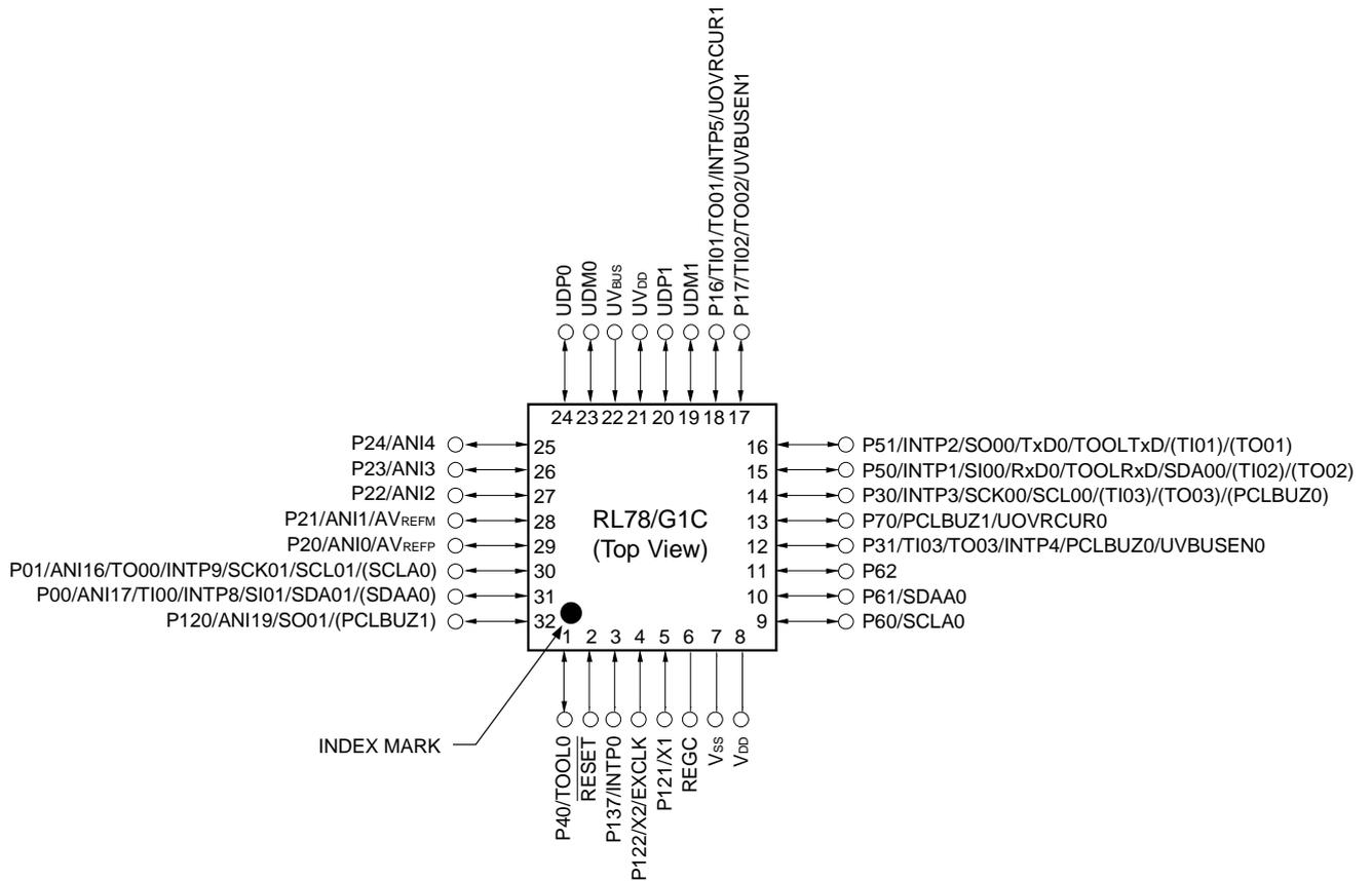
**Caution** Connect the REGC pin to V<sub>SS</sub> via a capacitor (0.47 to 1 μF).
