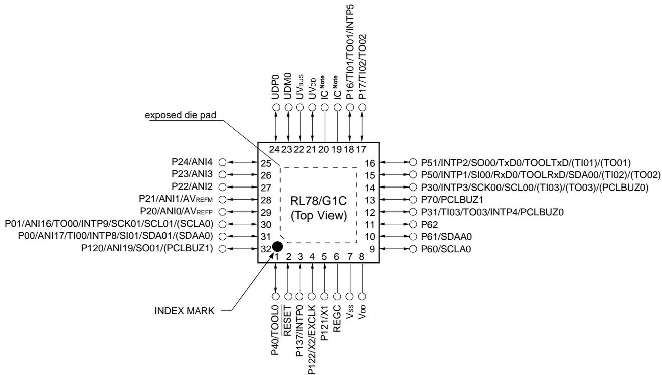
**Note** IC: Internal Connection Pin. Leave open.
