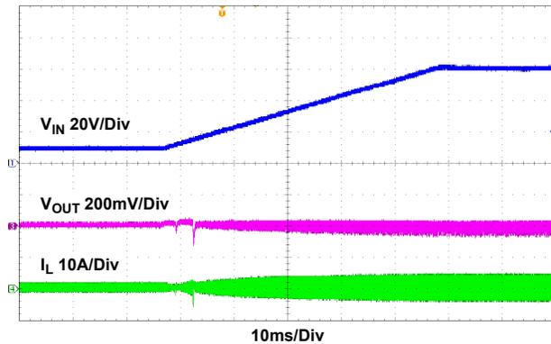
Figure 34. Line Transient,  $V_{IN} = 9V-60V$ ,  $1V/ms$ ,  $I_{OUT} = 0A$
