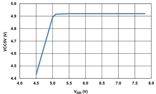
Figure 12.  $V_{CC5V}$  Line Regulation at 20mA Load
