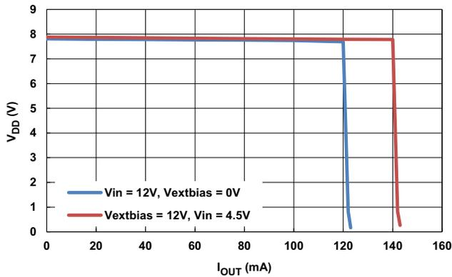
Figure 9.  $V_{DD}$  Load Regulation at 12V Input
