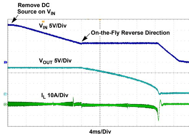
Figure 41. Bidirectional Operation
