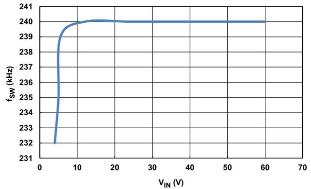
Figure 14. Switching Frequency vs  $V_{IN}$ ,  $R_T = 144k$
