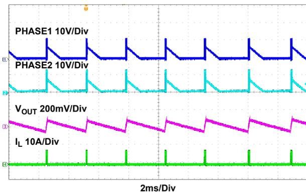
Figure 29. Burst Mode Waveforms,  $V_{IN} = 12V$ ,  $I_{OUT} = 0.1A$
