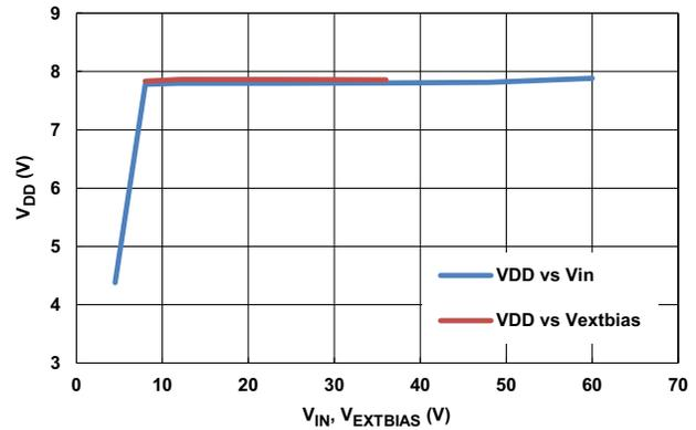
Figure 10.  $V_{DD}$  Line Regulation at 20mA Load
