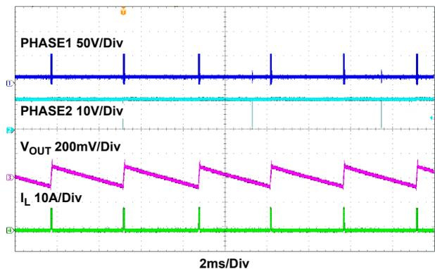
Figure 30. Burst Mode Waveforms,  $V_{IN} = 60V$ ,  $I_{OUT} = 0.1A$
