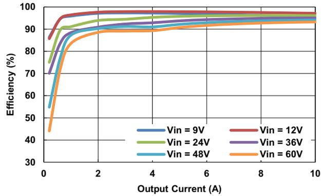
Figure 3. Efficiency ( $V_{OUT} = 12V$ , DE Mode)
