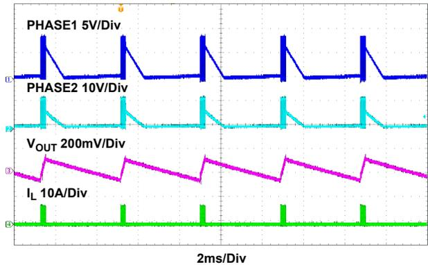
Figure 28. Burst Mode Waveforms,  $V_{IN} = 9V$ ,  $I_{OUT} = 0.1A$
