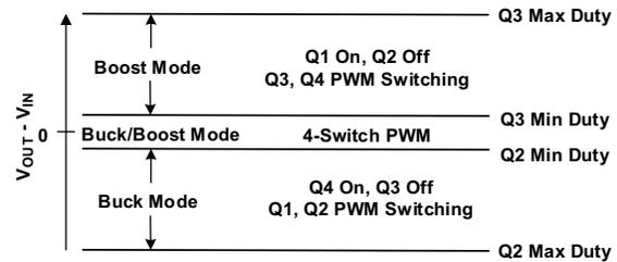
Figure 47. Operation Modes vs  $V_{OUT} - V_{IN}$
