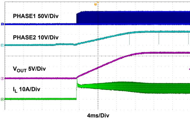
Figure 38. Start-Up Waveform,  $V_{IN} = 60V$   $I_O = 10A$ , CCM
