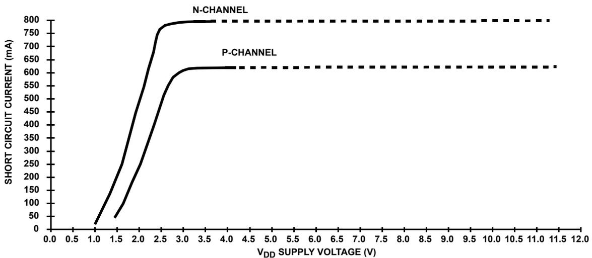
FIGURE 7. TYPICAL CHARACTERISTIC OF THE P AND N OUTPUT DRIVER SHORT CIRCUIT CURRENT vs SUPPLY VOLTAGE, T<sub>AMBIENT</sub> = 25°C
