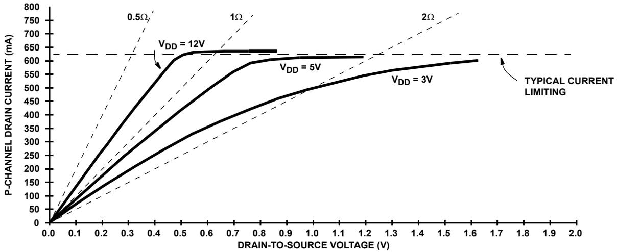
FIGURE 5. TYPICAL CHARACTERISTIC OF THE P-MOSFET OUTPUT DRIVER DRAIN CURRENT vs DRAIN-TO-SOURCE VOLTAGE, T<sub>AMBIENT</sub> = 25°C
