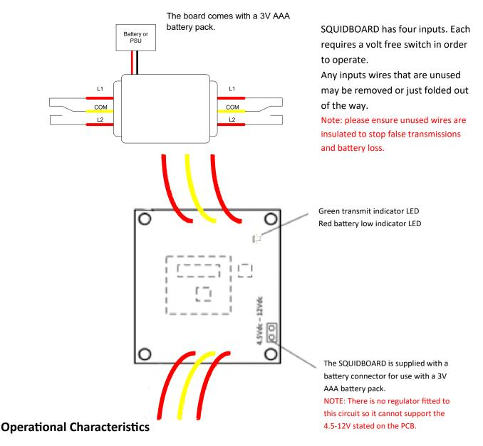
The SQUIDBOARD is very simple to connect and use. Simply wire a switch to any one or many of the inputs and send a signal.
