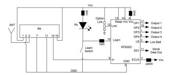
The Receiver application circuits generates a receiver decoder with four relay drive outputs and serial data output. It has easy Learn feature of the Keeloq transmitter and provides a Transmitter lower Battery indication.
