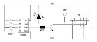
The transmitter application circuits generates a highly secure Keeloq protocol four switch transmitter encoder with LED indication or Transmission.
