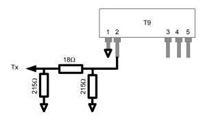
When laying out this network, keep all tracks as short as possible, especially ground paths and use 50 ohm track impedances when connecting to and from this network. This impedance can be realised on 1.6mm FR4 pcb by using a track width of 2.5mm.
