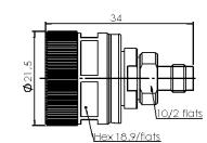
Part numberInterfaceR191 011 000PC7 - SMA Female33,7Image: state sta
