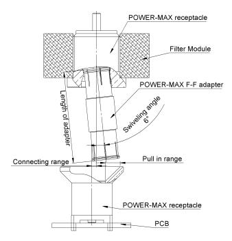
The connecting range represents the maximum misalignment during connection.
