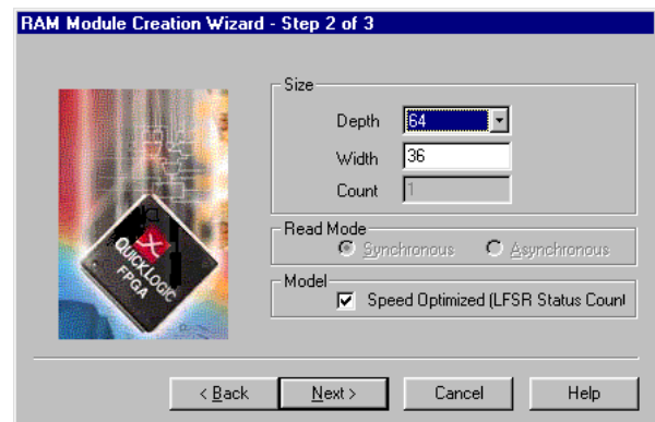
FIGURE 2. Graphical Interface to create FIFO
