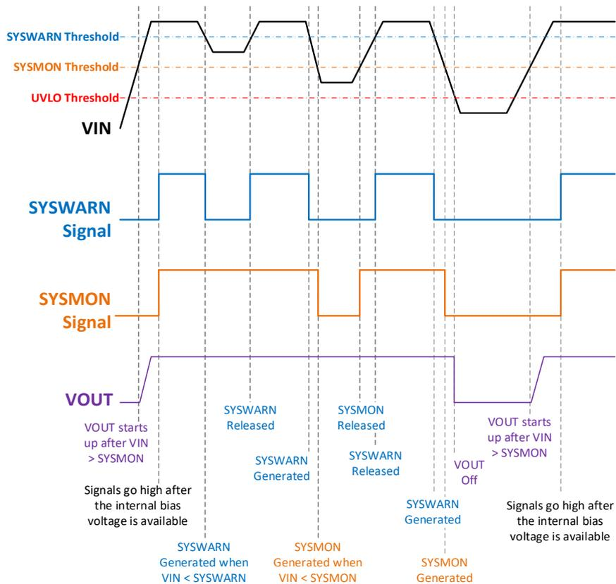
Figure 5: SYSMON and SYSWARN Signals
