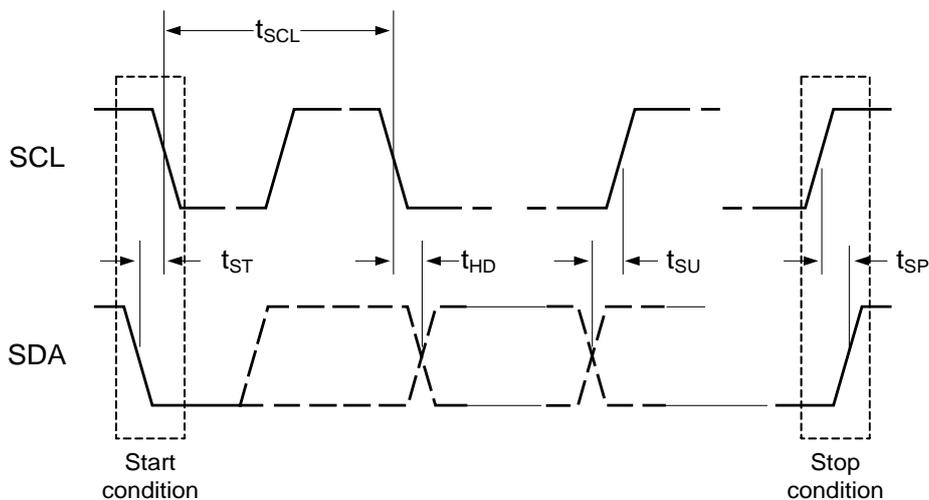
**Figure 2: I<sup>2</sup>C Data Transfer**
