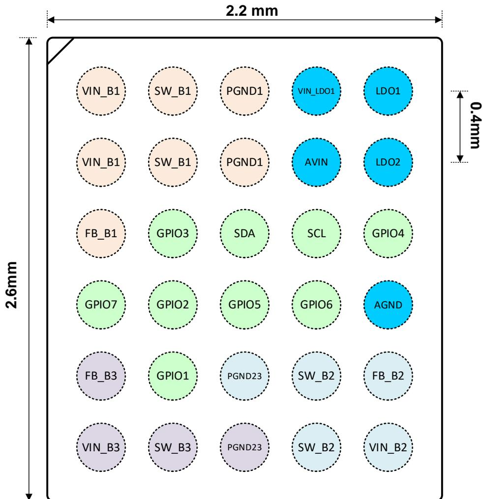
Figure 1: Pin Configuration – Top View (bumps down) – WLCSP- 30
