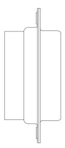
1. MATERIALS AND FINISHES: INSULATOR: GLASS FILLED POLYESTER PER ASTM-D5927, UL 94V-0, COLOR: BLUE. SHELLS: STEEL WITH TIN PLATE.
