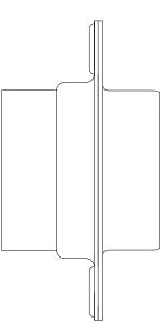
MATERIALS AND FINISHES: INSULATOR: GLASS FILLED POLYESTER PER ASTM D5927, UL 94Y-0, COLOR: BLUE. SHELLS: STEEL, TIN PLATE.
