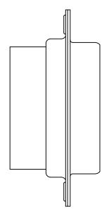
MATERIALS AND FINISHES: INSULATOR: GLASS FILLED DAP PER ASTM-D-5948, SDG-F, UL 94V-O, COLOR GREEN. SHELLS: STEEL, ZINC PLATE WITH CHROMATE SEAL.
