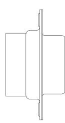
MATERIALS AND FINISHES: INSULATOR: GLASS FILLED DAP PER ASTM-D-5948, SDG-F, UL 94V-Q, GREEN COLOR. CONTACTS: PRECISION MACHINED COPPER ALLOY GOLD FLASH OVER NICKEL PLATE.
