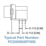
For right angle (90°) compliant press-fit contacts, specify code 62 in step 4 of ordering information.
