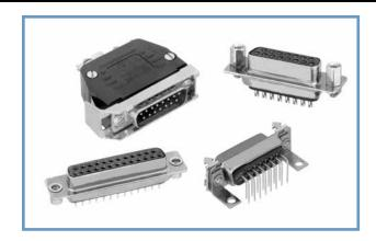
arrangements of 9, 15, 25, 37 and 50 contacts. Each Euro-D connector variant is available with contact terminations for solder cup, straight and right angle (90°) printed board mount terminations per standard European metric footprints. Euro-D series connectors are mateable and compatible with all D-subminiature connectors conforming to IEC 60807-2, IEC 60807-3 and MIL-DTL-24308.
