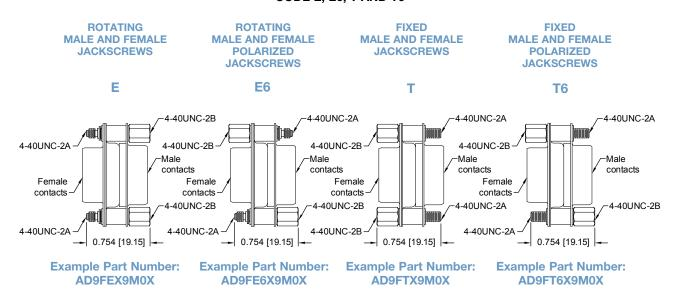
**MATERIAL:** Brass or steel with zinc plate and chromate seal or clear zinc plate or tin plate; stainless steel, passivated.
