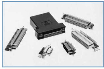
Five standard connector variants are offered in arrangements of 9, 15, 25, 37 and 50 contacts. Each connector variant is available with contact terminations for solder cup, straight and right angle (90°) printed board mount terminations with Inch and Metric footprints. Harmo-D series connectors are mateable and compatible with all D-subminiature connectors conforming to IEC 60807-2, IEC 60807-3 and MIL-DTL-24308.
