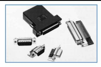
Six standard connector variants are offered in arrangements of 9, 15, 25, 37 and 50 contacts. Each Melo-D connector variant is available with contact terminations for solder cup, and straight and right angle (90°) printed board mount terminations featuring a choice of three printed board footprints. Melo-D series connectors are mateable and compatible with all D-subminiature connectors conforming to IEC 60807-2, IEC 60807-3 and MIL-DTL-24308.
