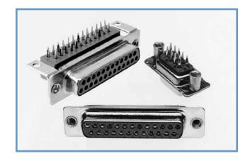
Five standard connector variants are offered in arrangement of 9, 15, 25, 37, and 50 contacts. PCD connectors are mateable and compatible with all D-subminiature connectors conforming to IEC 60807-2, IEC 60807-3, and dimensional requirements of MIL-DTL-24308.
