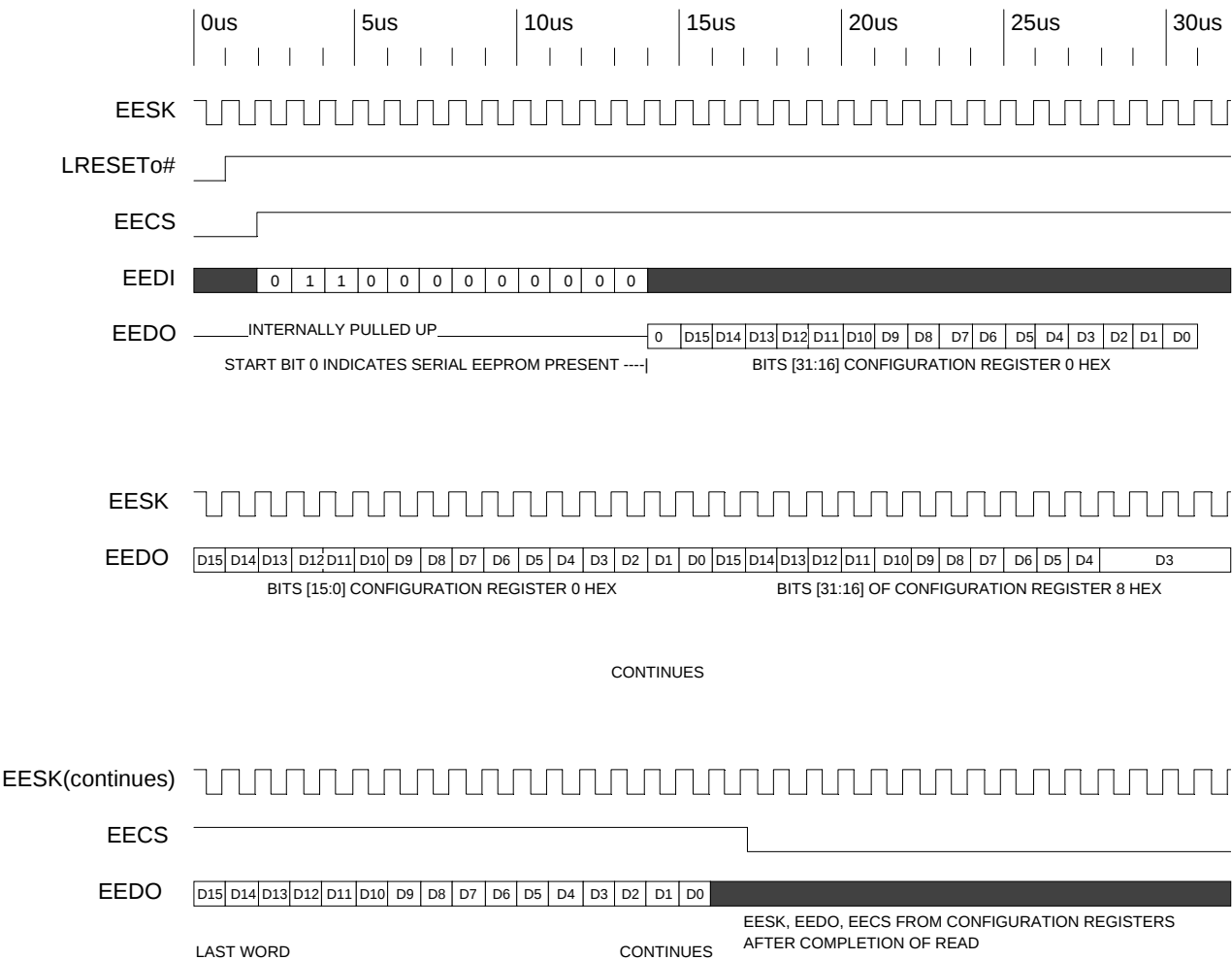
Timing Diagram 5-18. Initialization from Serial EEPROM (4K Bit)
