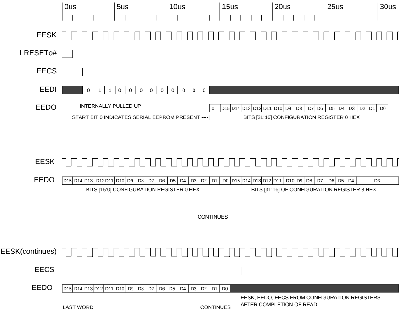
Timing Diagram 3-27. Initialization from Serial EEPROM (4K Bit)
