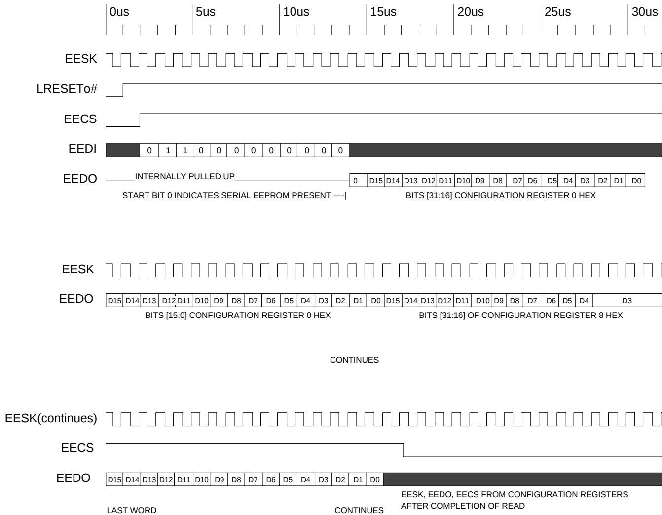
Timing Diagram 2-2. Initialization from Serial EEPROM (4K Bit)
