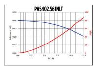
High Current Molded Power Inductor - PA5402 & PM5402 Series
