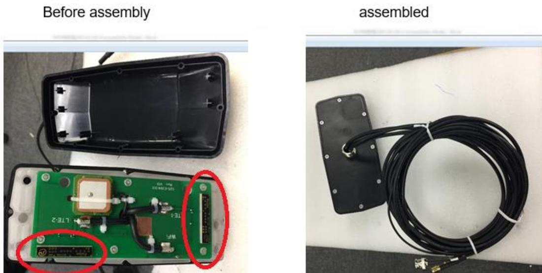
Test Method: The whole assembly at 1 meter drop. A minimum of one drop per orientation - flat top, bottom, side and corner (a total of 4 drops). It's recommended to get one drop on flat top, bottom, all four flat sides and four top corners, a total of 10 drops. (Note: MIL STD and JASO D001-1994 cites to drop products on a 2 inch plywood backed by concrete floor)
