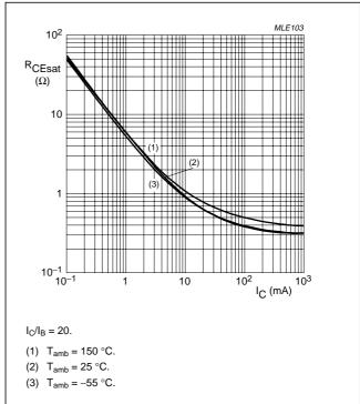
Fig.7 Collector-emitter equivalent on-resistance as a function of collector current; typical values.
