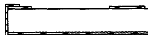
"R" OR "B" TERMINATION FRONT & BACK SIDE METAL WRAPAROUND ON SHUNT CONNECTION ONLY
