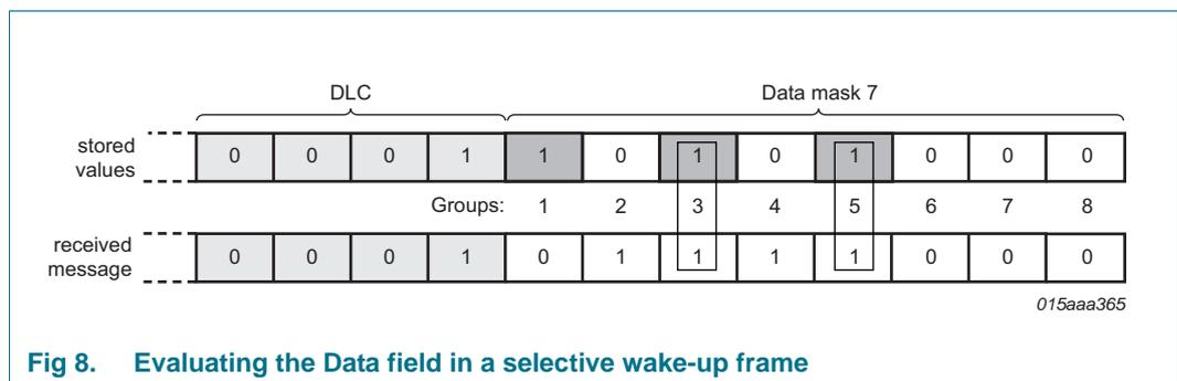
Optionally, the data length code and the data field can be excluded from the evaluation of the wake-up frame. If bit PNDM = 0, only the identifier field is evaluated to determine if the frame contains a valid wake-up message. If PNDM = 1 (the default value), the data field is included as part of the wake-up filtering.
