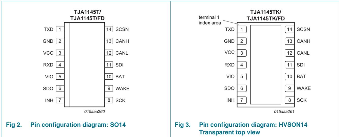
Fig 2. Pin configuration diagram: SO14
