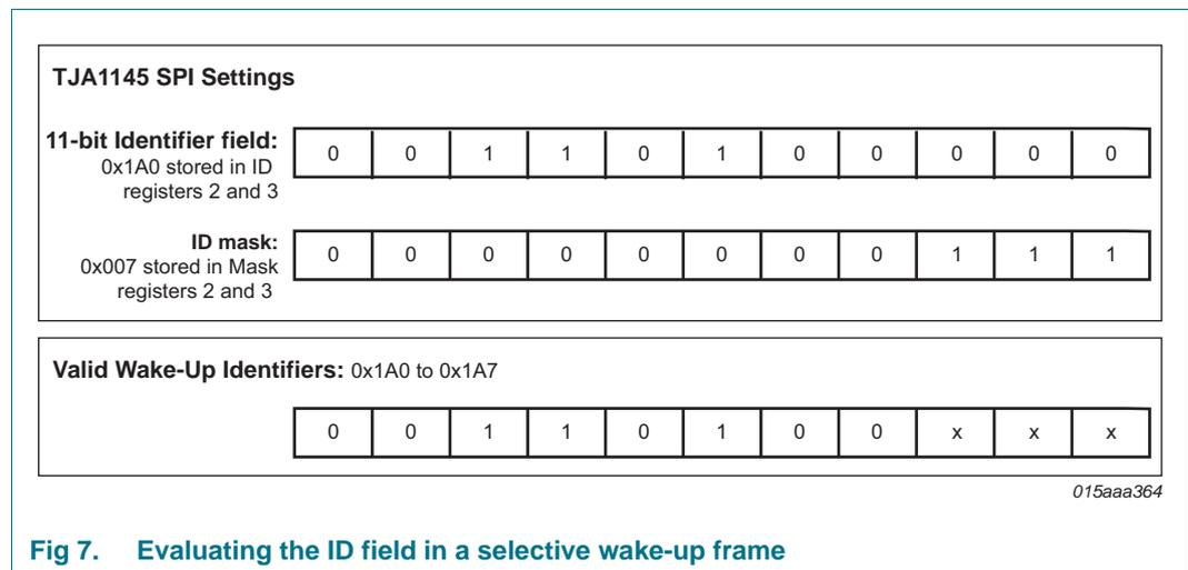
The data field indicates which nodes are to be woken up. Groups of nodes can be pre-defined and associated with bits in a data mask. By comparing the incoming data field with the data mask, multiple groups of nodes can be woken up by a single wake-up message.
