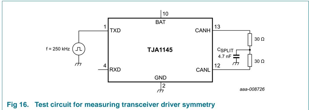
Fig 16. Test circuit for measuring transceiver driver symmetry
