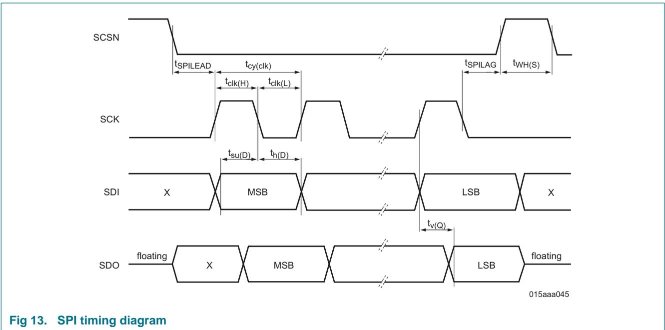
Fig 13. SPI timing diagram
