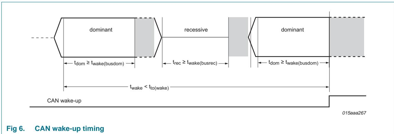
Fig 6. CAN wake-up timing
