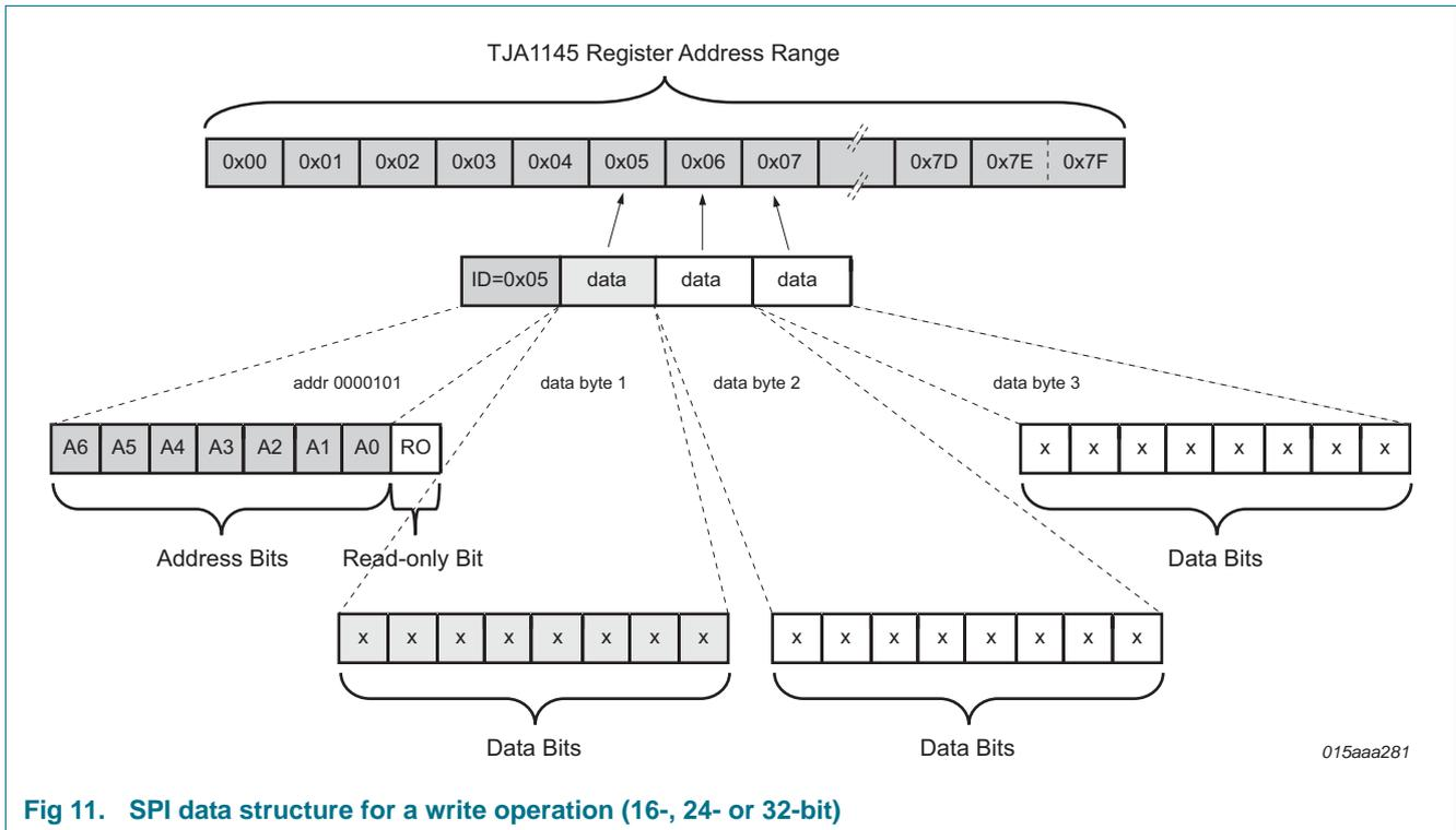
**Fig 11. SPI data structure for a write operation (16-, 24- or 32-bit)**
