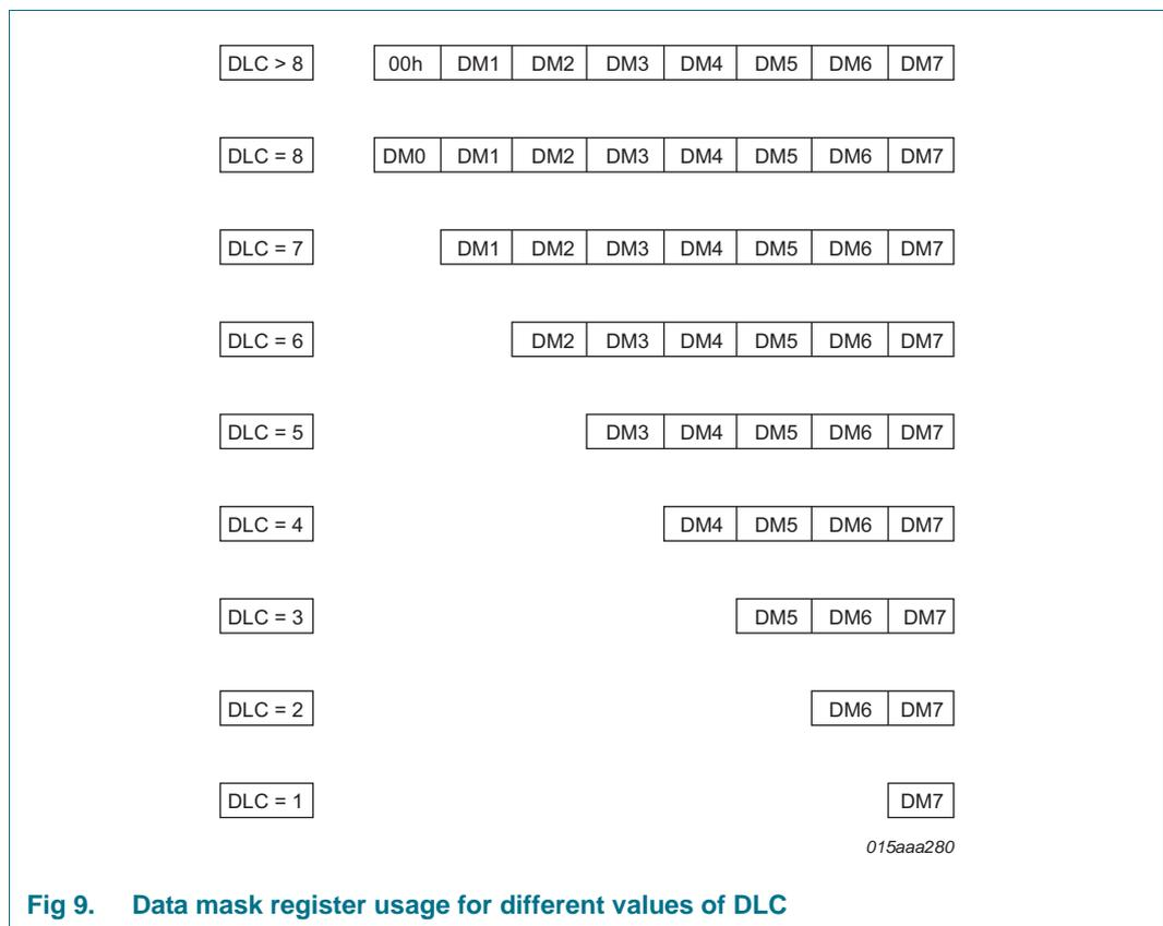
**Fig 9. Data mask register usage for different values of DLC**
