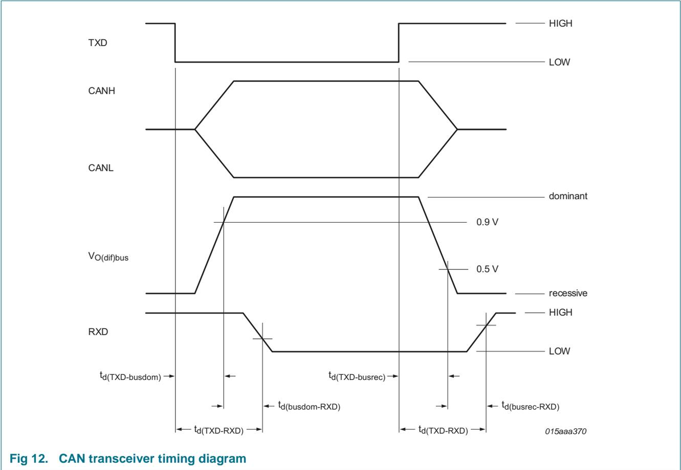
Fig 12. CAN transceiver timing diagram
