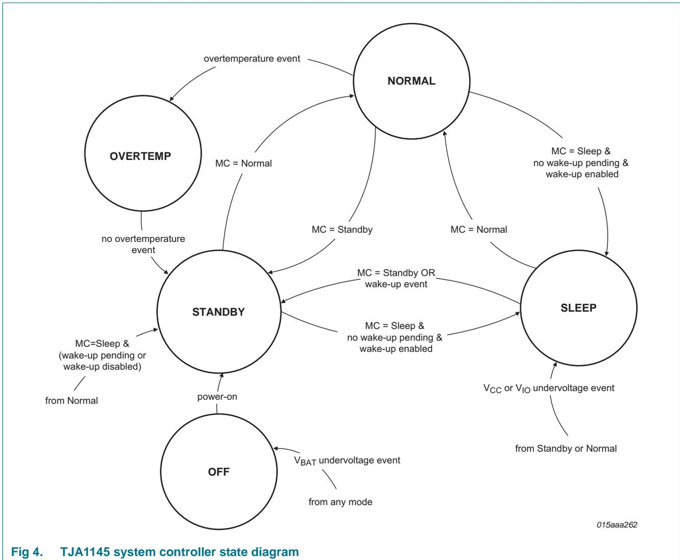
Fig 4. TJA1145 system controller state diagram
