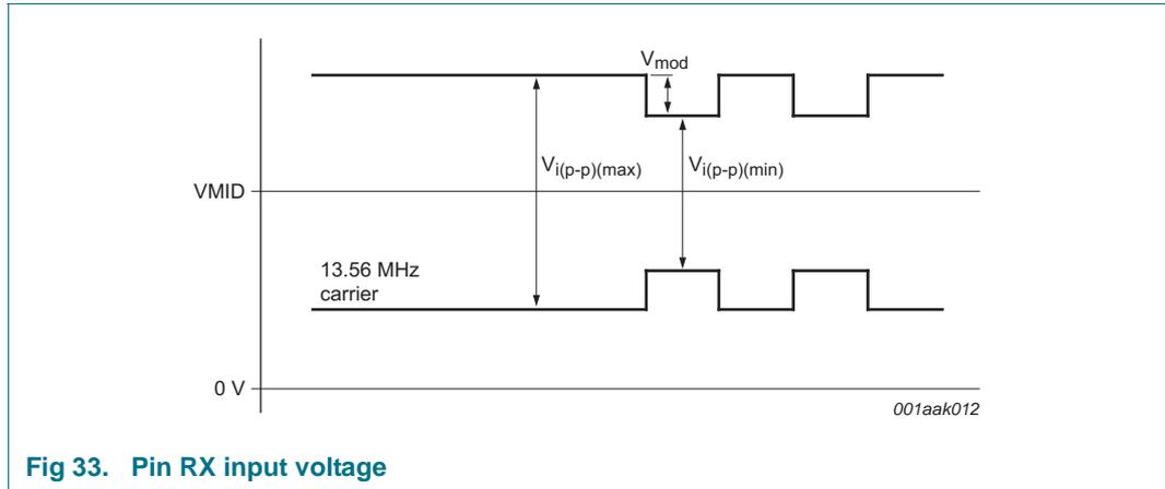
Fig 33. Pin RX input voltage
