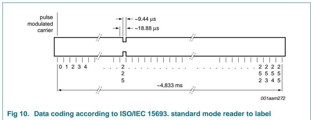
**Fig 10. Data coding according to ISO/IEC 15693. standard mode reader to label**
