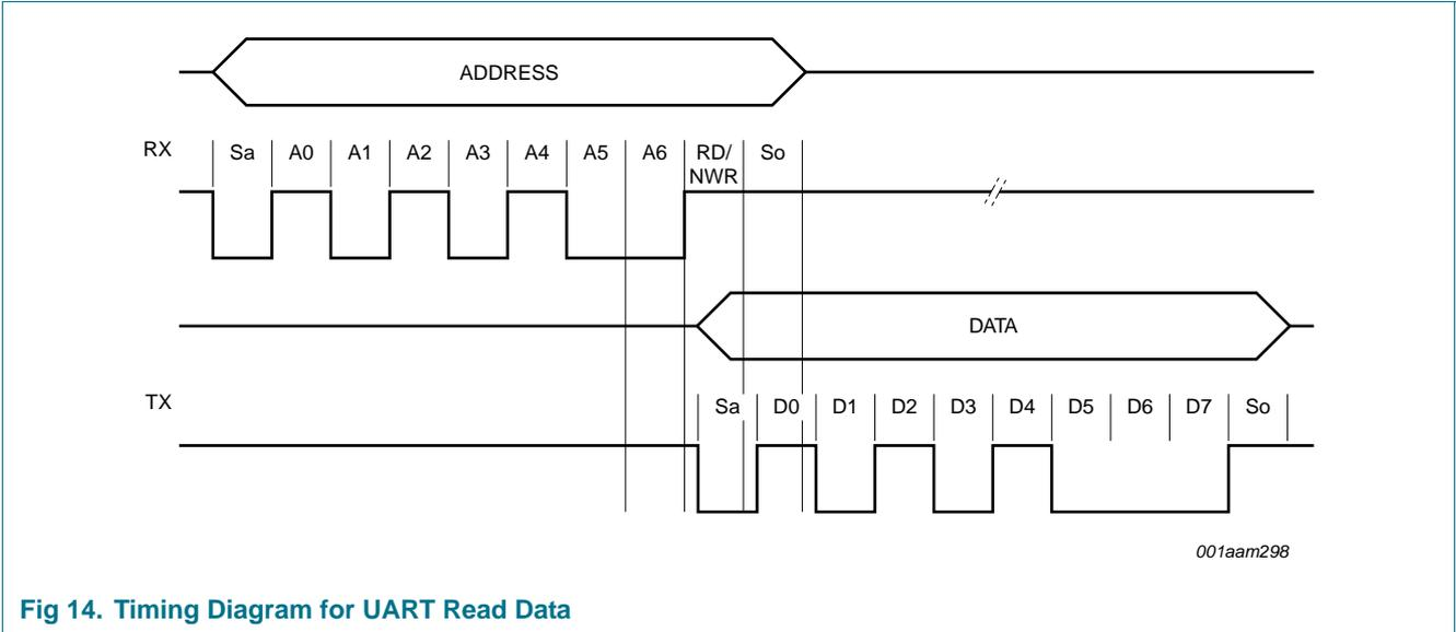
Fig 14. Timing Diagram for UART Read Data
