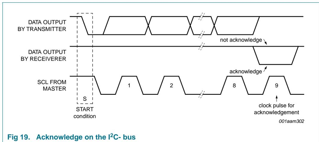
Fig 19. Acknowledge on the I<sup>2</sup>C- bus
