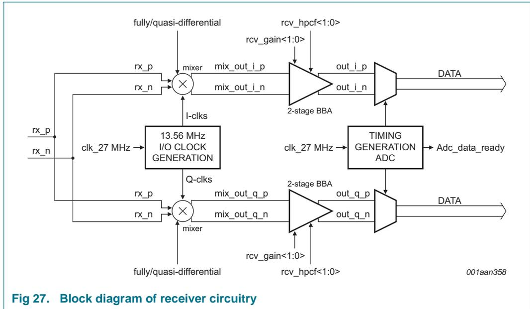
Fig 27. Block diagram of receiver circuitry
