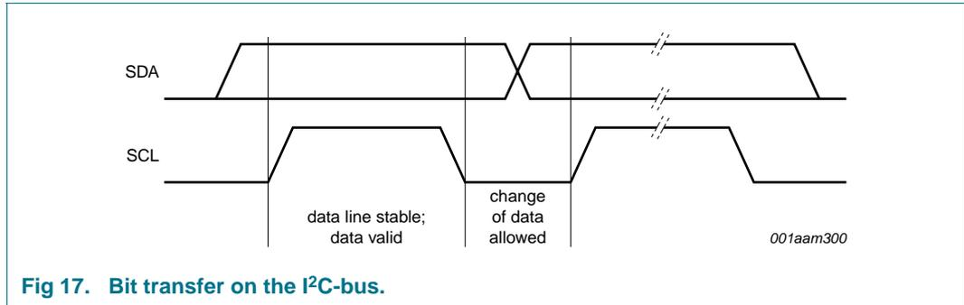
Fig 17. Bit transfer on the I<sup>2</sup>C-bus.
