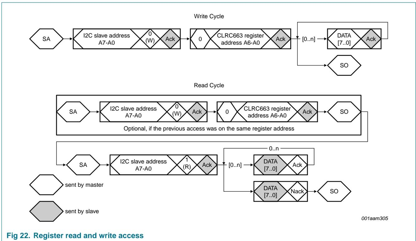
Fig 22. Register read and write access
