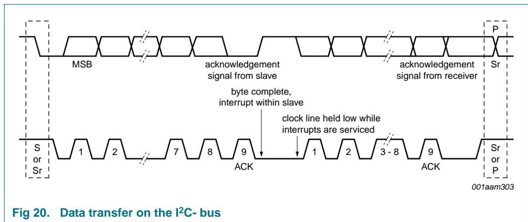
Fig 20. Data transfer on the I<sup>2</sup>C- bus
