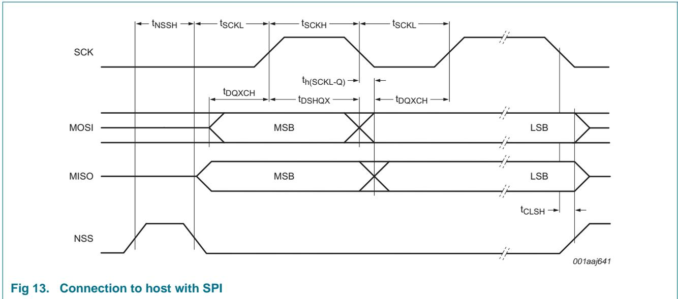
Fig 13. Connection to host with SPI
