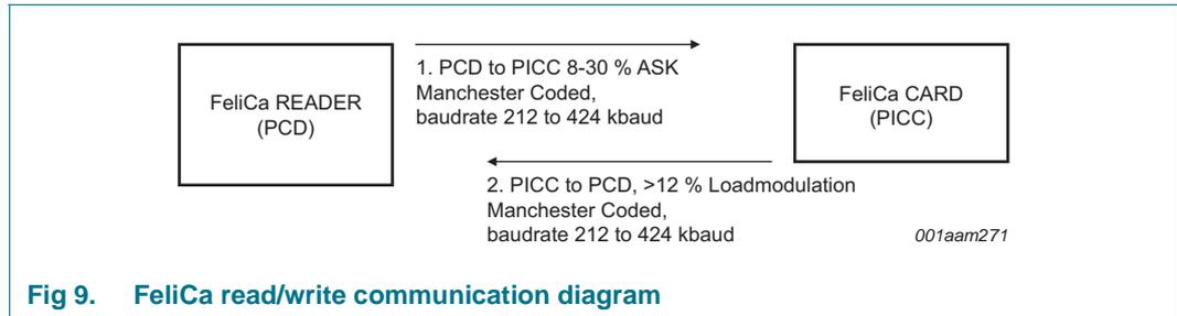
Fig 9. FeliCa read/write communication diagram
