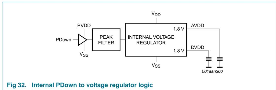
**Fig 32. Internal PDown to voltage regulator logic**
