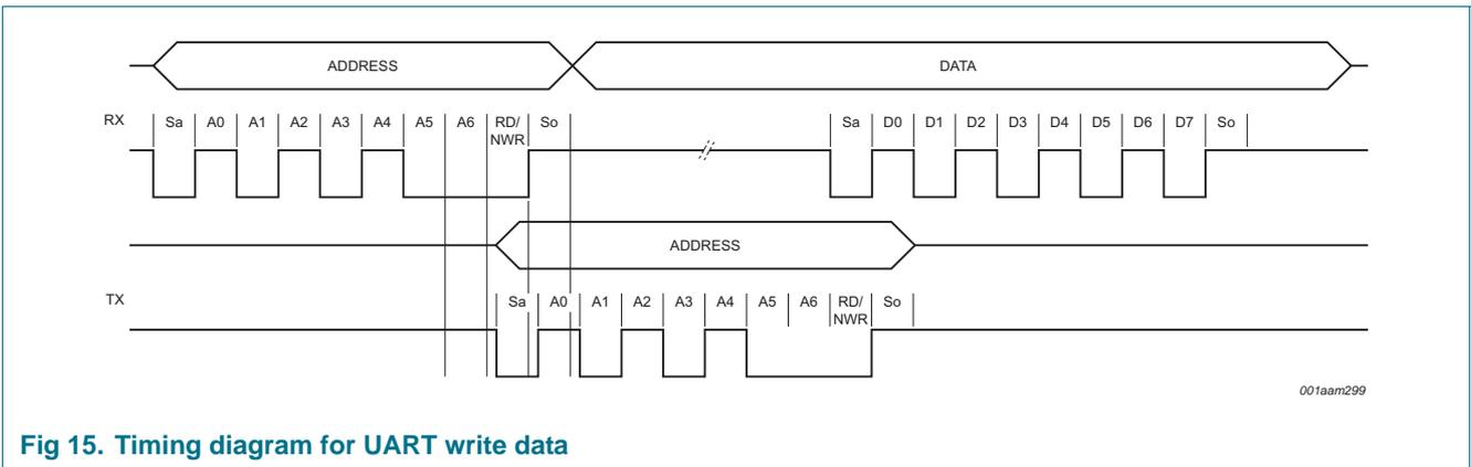
Fig 15. Timing diagram for UART write data
