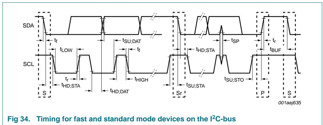
Fig 34. Timing for fast and standard mode devices on the I<sup>2</sup>C-bus
