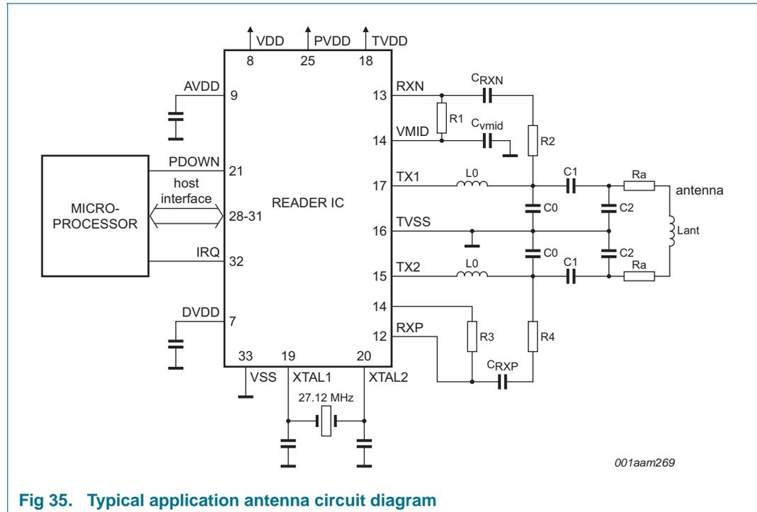
Fig 35. Typical application antenna circuit diagram
