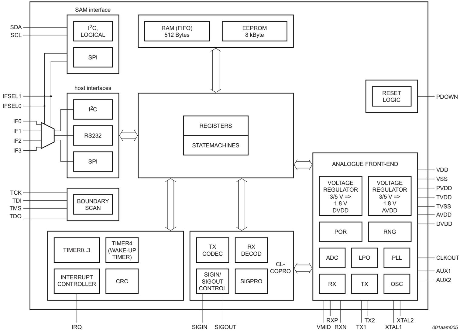
Fig 3. Detailed block diagram of the CLRC663
