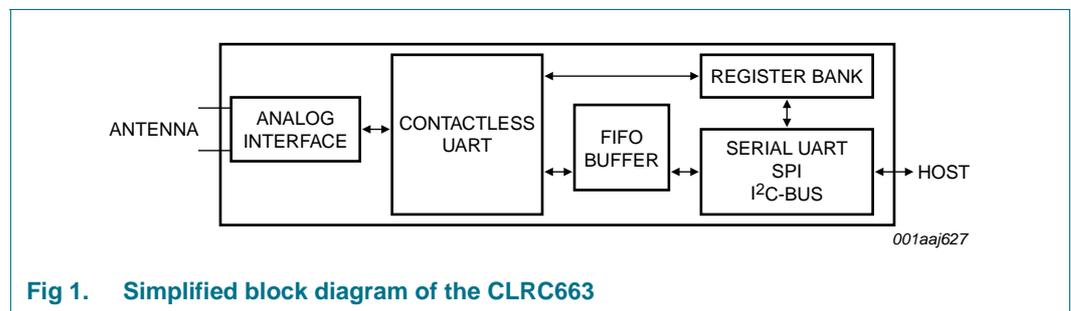
Fig 1. Simplified block diagram of the CLRC663
