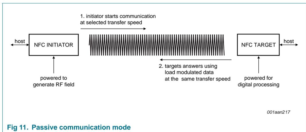
**Fig 11. Passive communication mode**
