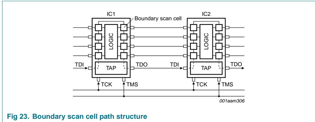
Fig 23. Boundary scan cell path structure
