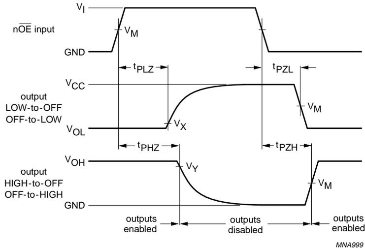
$V_M = 0.5V_{CC}$  at  $V_{CC} < 2.7\text{ V}$  and  $V_M = 1.5\text{ V}$  at  $V_{CC} \geq 2.7\text{ V}$ .
