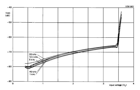
Fig. 9 Input signal handling capability; gain = -10 dB; R<sub>S</sub> =  $600~\Omega$ ; R<sub>L</sub> =  $10~k\Omega$ ; bass/trebble = 0~dB; V<sub>CC</sub> = 12~V.
