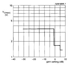
Fig. 10 Input signal handling capacility plotted against gain setting; THD = -60 dB; f = 1 kHz; R<sub>S</sub> =  $600~\Omega$ ; R<sub>L</sub> =  $10~k\Omega$ ; bass/trebble = 0 dB; V<sub>CC</sub> = 12~V.
