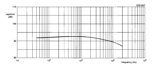
Fig. 14 Mute signal rejection as a function of frequency; gain = 0 dB;  $V_i$  = 1.0 V;  $R_S$  = 0  $\Omega$ ;  $R_L$  = 10 k $\Omega$ ; bass/trebble = 0 dB;  $V_{CC}$  = 12 V.
