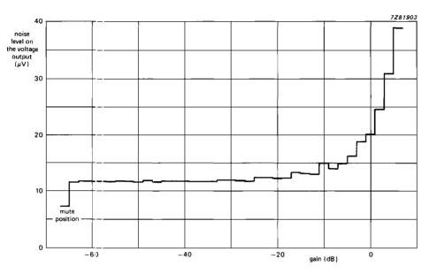
Fig. 16 Noise output voltage as a function of gain; weighted CCIR468 quasi peak gain, + 6 dB to -64 dB;  $V_i$  = 0 V,  $R_S$  = 0  $\Omega$ ;  $R_{\perp}$  = 10 k $\Omega$ ; bass/trebble = 0 dB;  $V_{CC}$  = 12 V.
