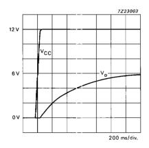
Fig. 20 Turn-on behaviour;  $C = 2.2 \mu F$ ;  $R_L = 10 k\Omega$ .
