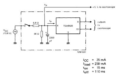
Fig. 23 Turn-on/off power supply circuit diagram.
