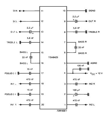
Fig. 25 Test and application circuit diagram.
