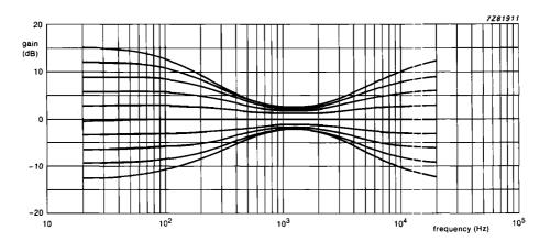
Fig. 18 Tone control with T-filter.
