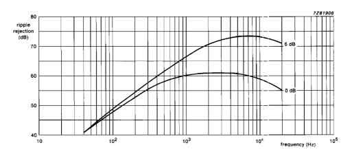
Fig. 15 Ripple rejection as a function of frequency; voltage ripple = 0.3 V (rms); R<sub>S</sub> = 0  $\Omega$ , R<sub>L</sub> = 10 k $\Omega$ ; bass/trebble = 0 dB; V<sub>CC</sub> = 12 V.
