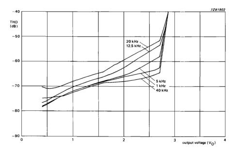
Fig. 11 Output signal handling capability; gain = 6 dB; R<sub>S</sub> = 600  $\Omega$ ; R<sub>L</sub> = 10 k $\Omega$ , bass/trebble = 0 dB, V<sub>CC</sub> = 12 V.
