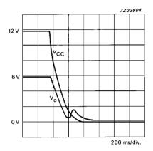
Fig. 21 Turn-off behaviour; without modulation.
