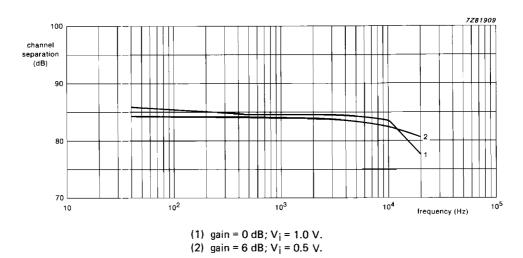
Fig. 13 Stereo channel separation as a function of frequency; R<sub>S</sub> = 0  $\Omega$ , R<sub>L</sub> = 10 k $\Omega$ ; bass/trebble = 0 dB; V<sub>CC</sub> = 12 V.
