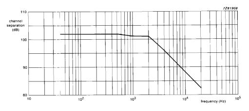
Fig. 12 Source selector separation (channel 2 and channel 1); gain = 0 dB;  $V_{i1}$  = 0 V;  $V_{i2}$  = 1 V,  $R_S$  = 0  $\Omega$ ;  $R_L$  = 10 k $\Omega$ ; pass/trebble = 0 dB;  $V_{CC}$  = 12 V.
