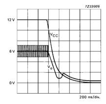
Fig. 22 Turn-off behaviour; with modulation (shaded area).
