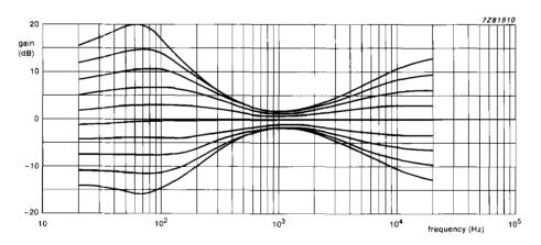
Fig. 17 Frequency response of bass and trebble control; bass and trebble gain settings = -12 to + 15 dB; gain is 0 dB;  $V_i$  = 0.1 V;  $R_{S9}$  = 600  $\Omega$ ;  $R_L$  = 10 k $\Omega$ ;  $V_{CC}$  = 12 V.
