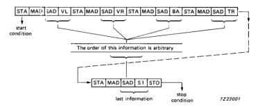
Fig. 4 Data transmission after a power-on reset.
