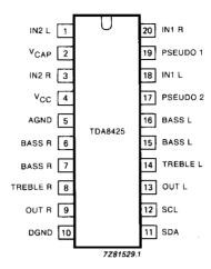
Fig. 2 Pinning diagram.
