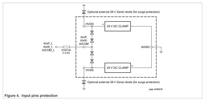
Each HV input pin is equipped with input protection diodes connected to HVDD, HVSS.
