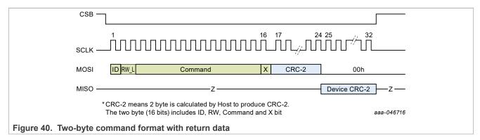
**Two-byte command:** Two-byte command format with data return.
