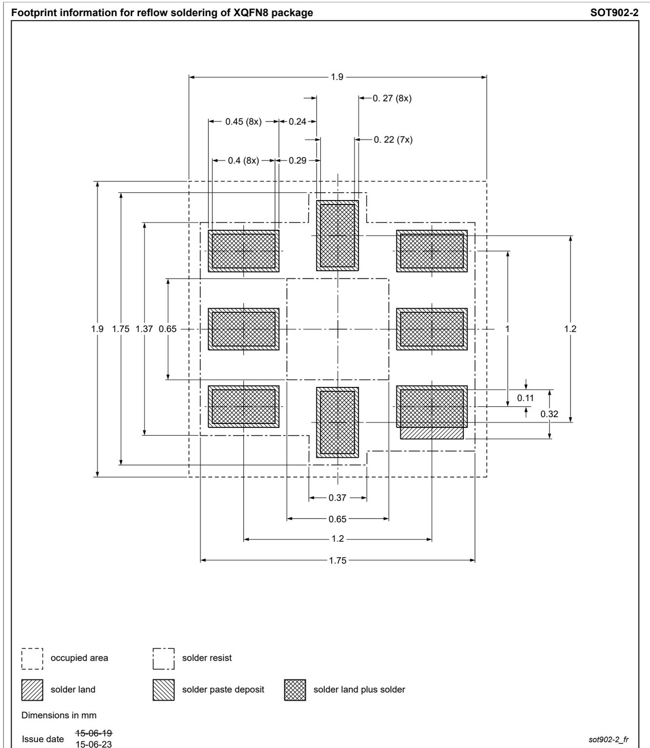
Figure 27. PCB footprint for SOT902-2 (XQFN8); reflow soldering
