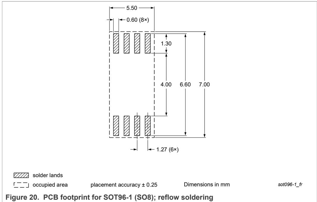
Figure 20. PCB footprint for SOT96-1 (SO8); reflow soldering
