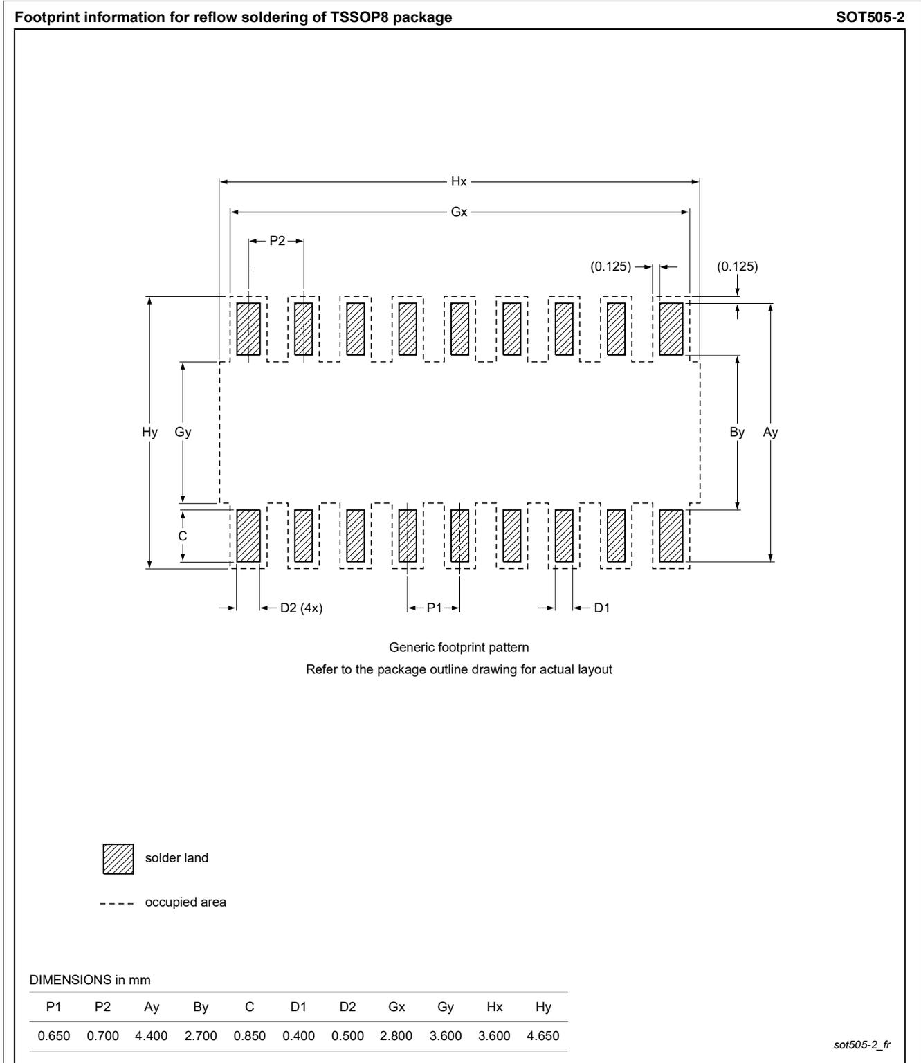
Figure 23. PCB footprint for SOT505-2 (TSSOP8); reflow soldering
