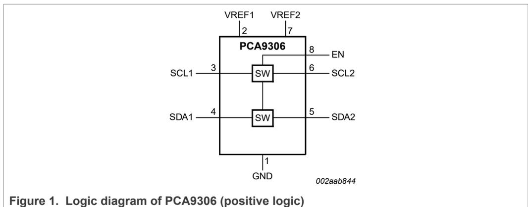
Figure 1. Logic diagram of PCA9306 (positive logic)
