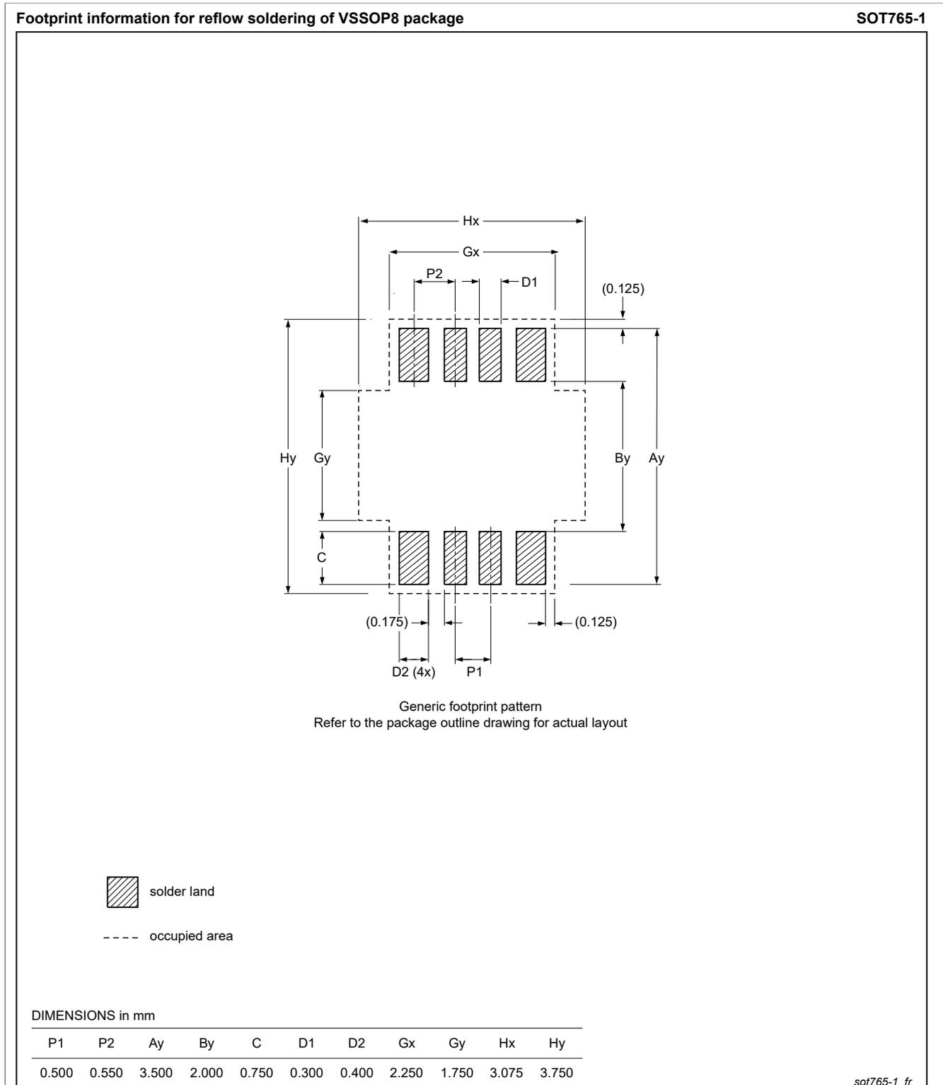
Figure 24. PCB footprint for SOT765-1 (VSSOP8); reflow soldering
