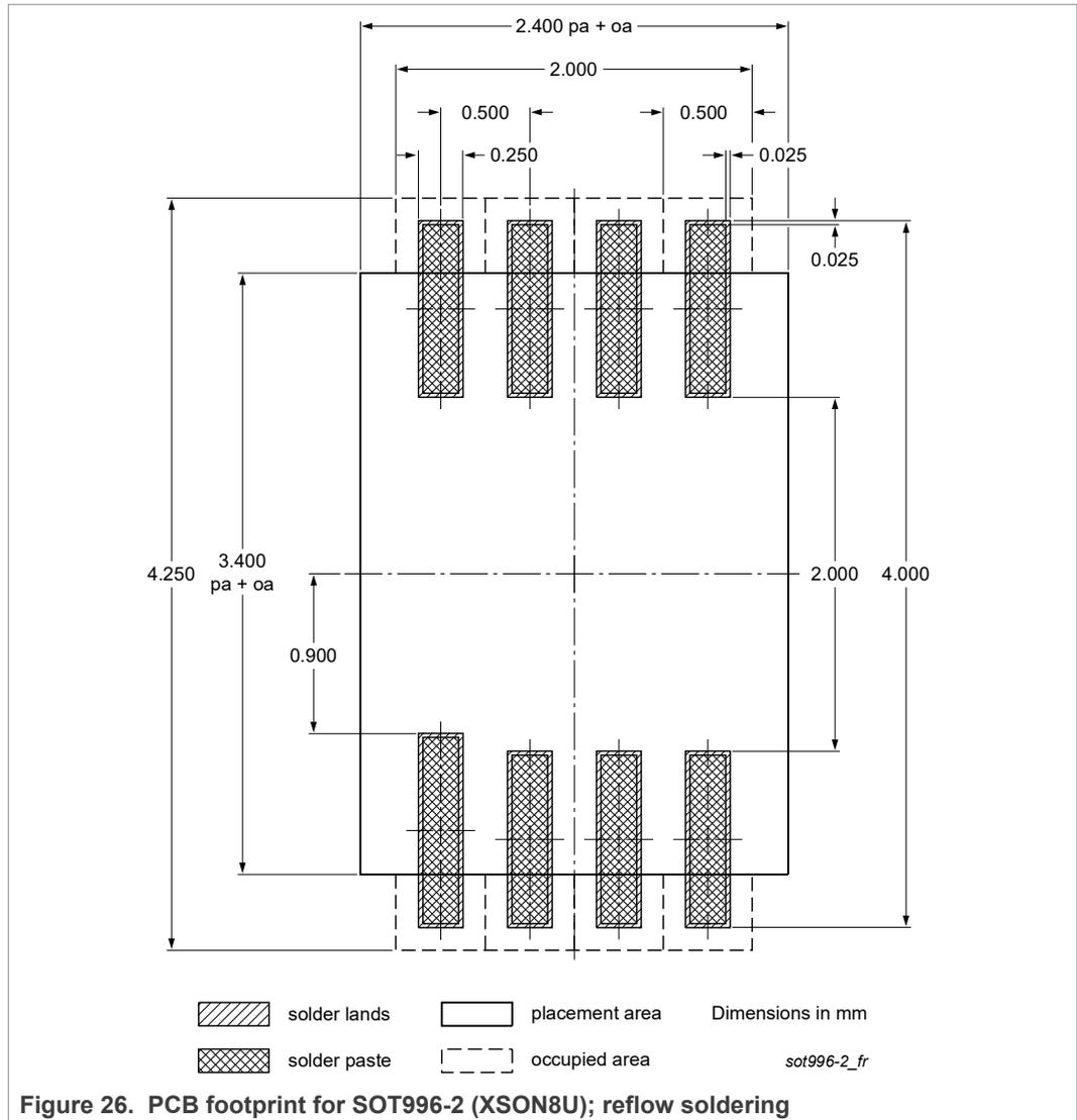
Figure 26. PCB footprint for SOT996-2 (XSON8U); reflow soldering
