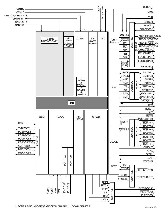
Figure 3-1 MC68336/376 Block Diagram
