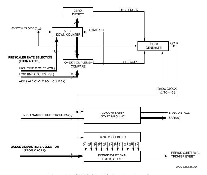
Figure 8-8 QADC Clock Subsystem Functions
