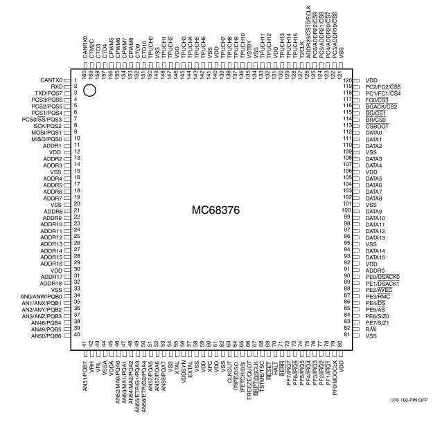
Figure 3-3 MC68376 Pin Assignments for 160-Pin Package
