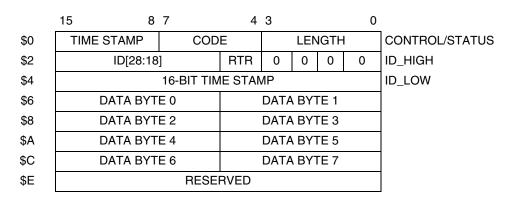
Figure 13-4 Standard ID Message Buffer Structure
