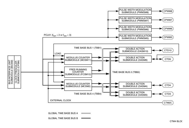
Figure 10-1 CTM4 Block Diagram
