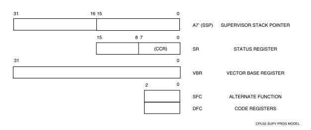
Figure D-2 Supervisor Programming Model Supplement
