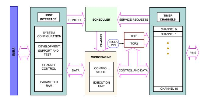
Figure 11-1 TPU Block Diagram
