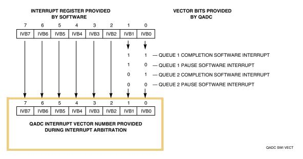
Figure 8-11 QADC Interrupt Vector Format
