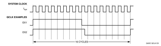
Figure 8-9 QADC Clock Programmability Examples
