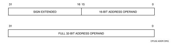
Figure 4-5 Address Organization in Address Registers
