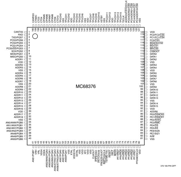
Figure B-2 MC68376 Pin Assignments for 160-Pin Package
