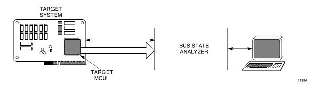
Figure 4-9 Bus State Analyzer Configuration
