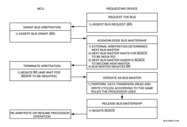
Figure 5-15 Bus Arbitration Flowchart for Single Request
