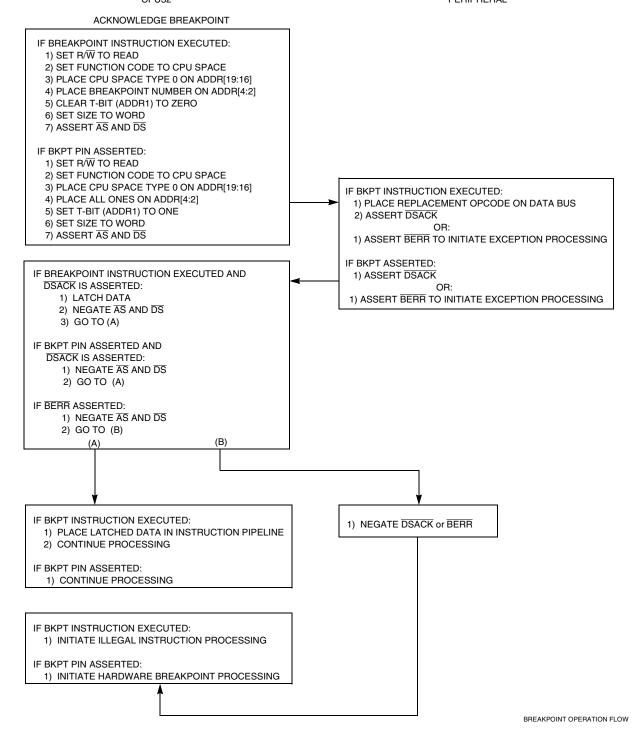
Figure 5-13 Breakpoint Operation Flowchart
