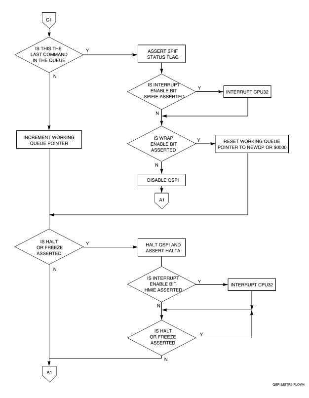
Figure 9-7 Flowchart of QSPI Master Operation (Part 3)
