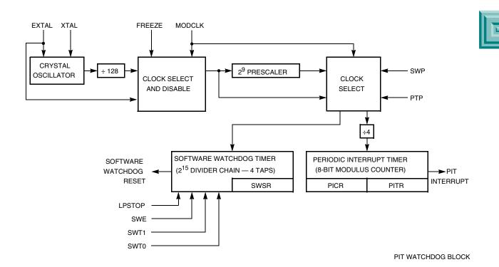
Figure 5-7 Periodic Interrupt Timer and Software Watchdog Timer
