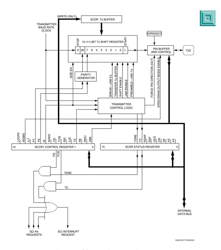
Figure 9-10 SCI Transmitter Block Diagram
