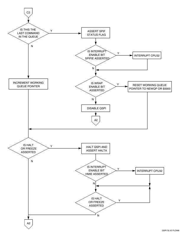
Figure 9-9 Flowchart of QSPI Slave Operation (Part 2)
