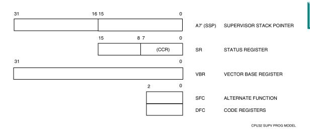
Figure 4-3 Supervisor Programming Model Supplement
