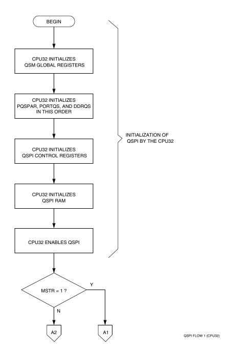
Figure 9-4 Flowchart of QSPI Initialization Operation
