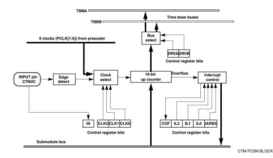
Figure 10-3 FCSM Block Diagram
