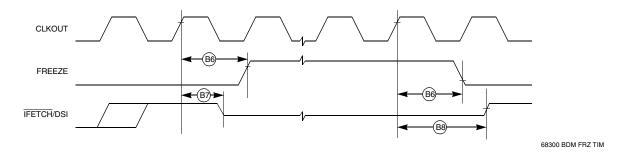
Figure A-14 Background Debugging Mode Timing — Freeze Assertion
