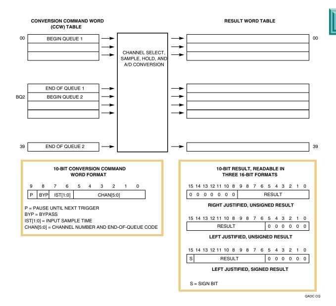
Figure 8-10 QADC Conversion Queue Operation
