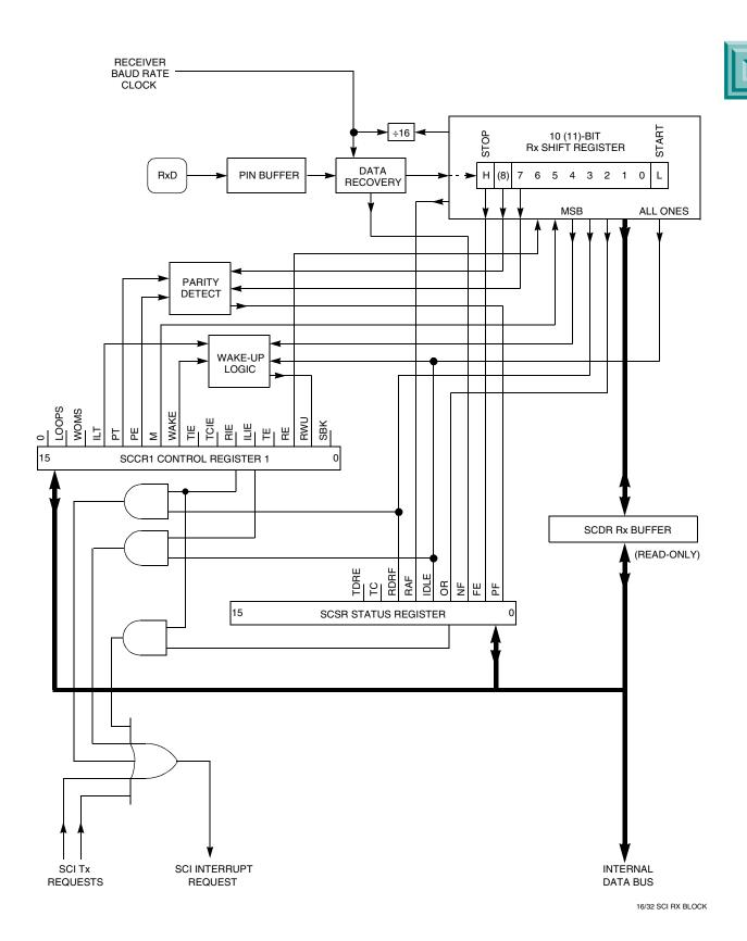
Figure 9-11 SCI Receiver Block Diagram
