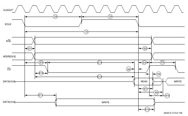
Figure A-15 ECLK Timing Diagram
