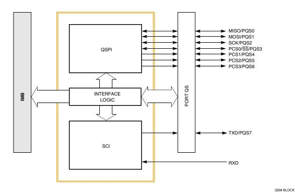
Figure 9-1 QSM Block Diagram
