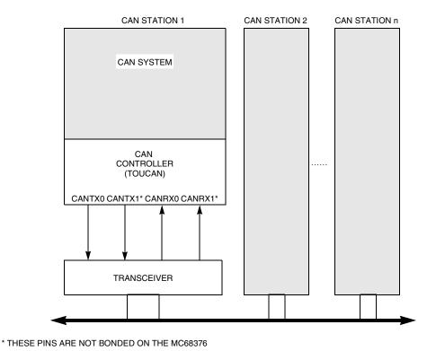
Figure 13-2 Typical CAN Network
