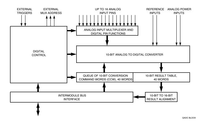
Figure 8-1 QADC Block Diagram
