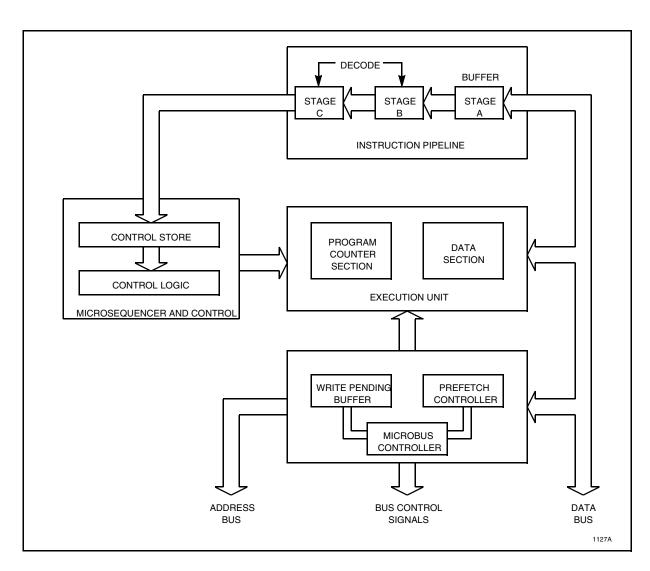
Figure 4-1 CPU32 Block Diagram
