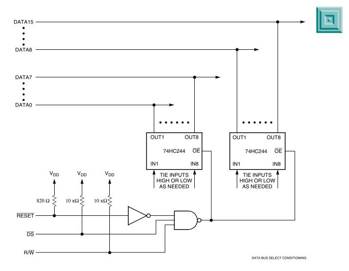
Figure 5-16 Preferred Circuit for Data Bus Mode Select Conditioning
