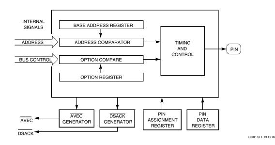
Figure 5-20 Chip-Select Circuit Block Diagram
