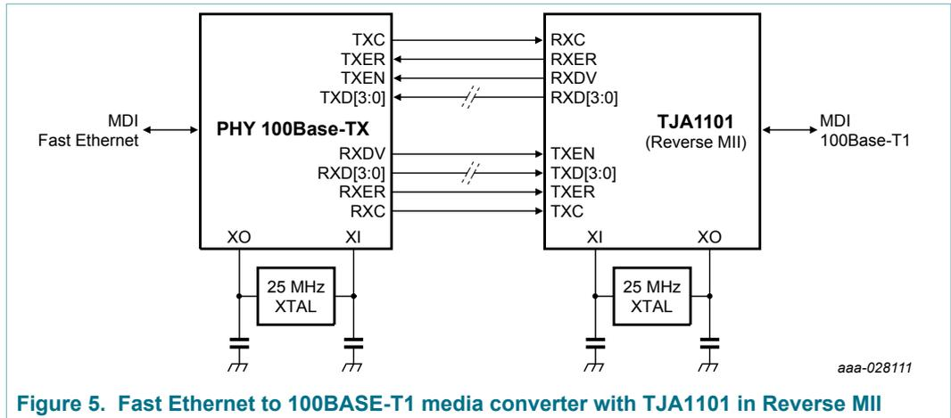
Figure 5. Fast Ethernet to 100BASE-T1 media converter with TJA1101 in Reverse MII
