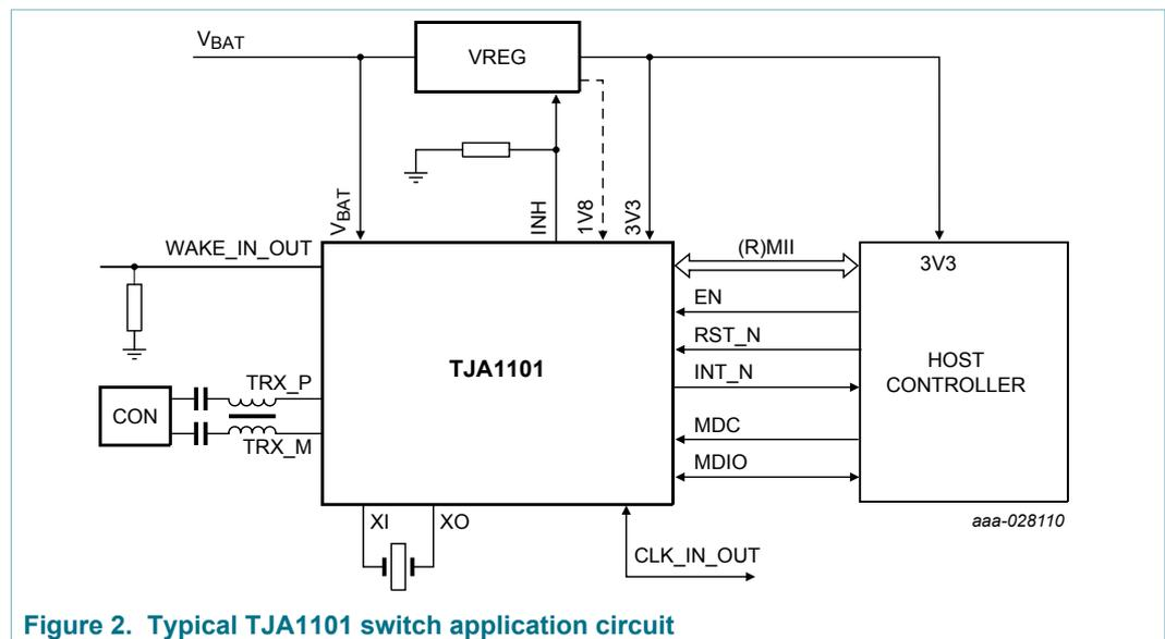
Figure 2. Typical TJA1101 switch application circuit
