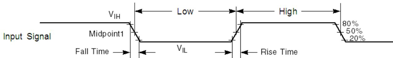
The midpoint is  $V_{IL} + (V_{IH} - V_{IL})/2$ .
