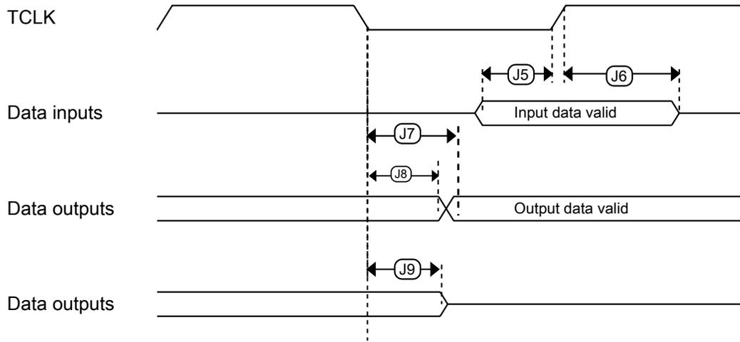
Figure 33. Boundary scan (JTAG) timing
