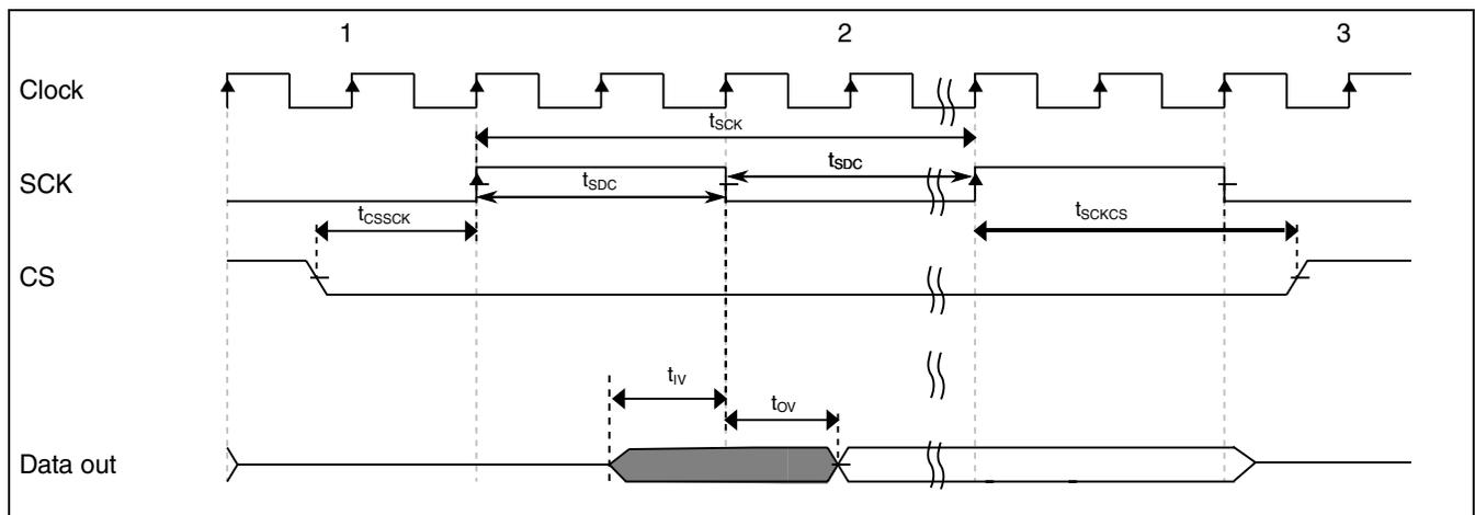
Figure 10. QuadSPI output timing (SDR mode) diagram
