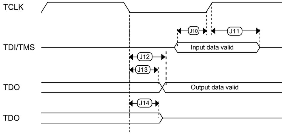
Figure 34. Test Access Port timing
