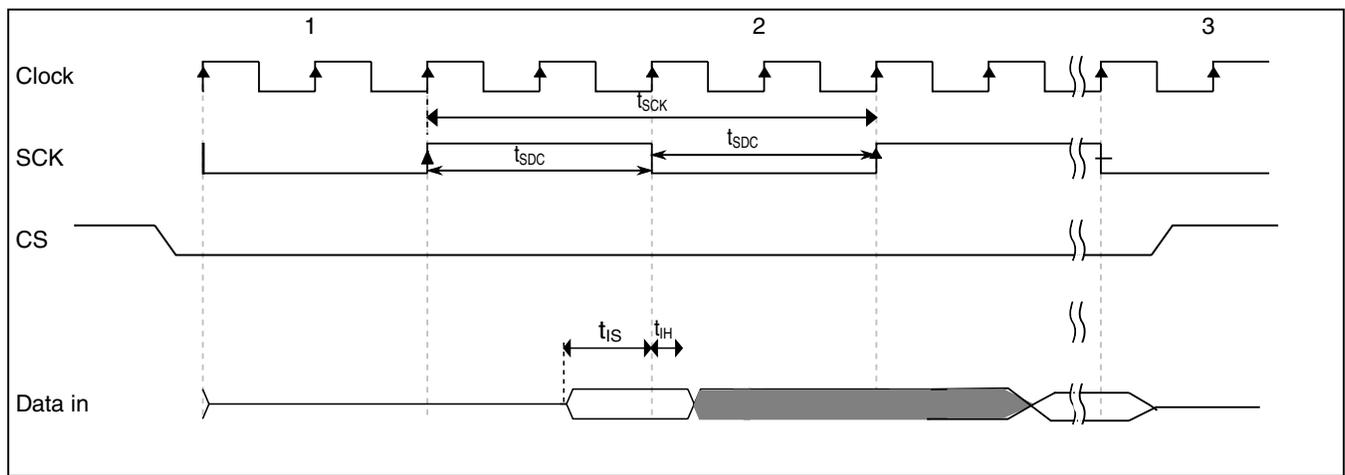
Figure 9. QuadSPI input timing (SDR mode) diagram
