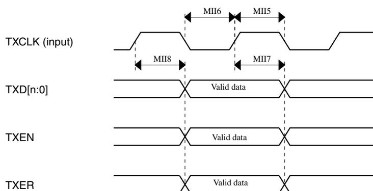
Figure 25. MII transmit signal diagram
