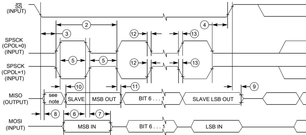
Figure 21. LPSPI slave mode timing (CPHA = 1)
