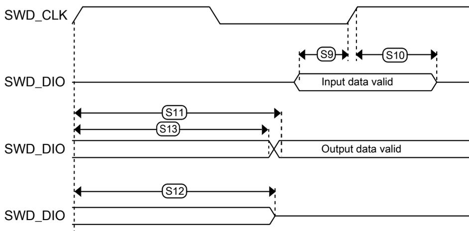
Figure 30. Serial wire data timing
