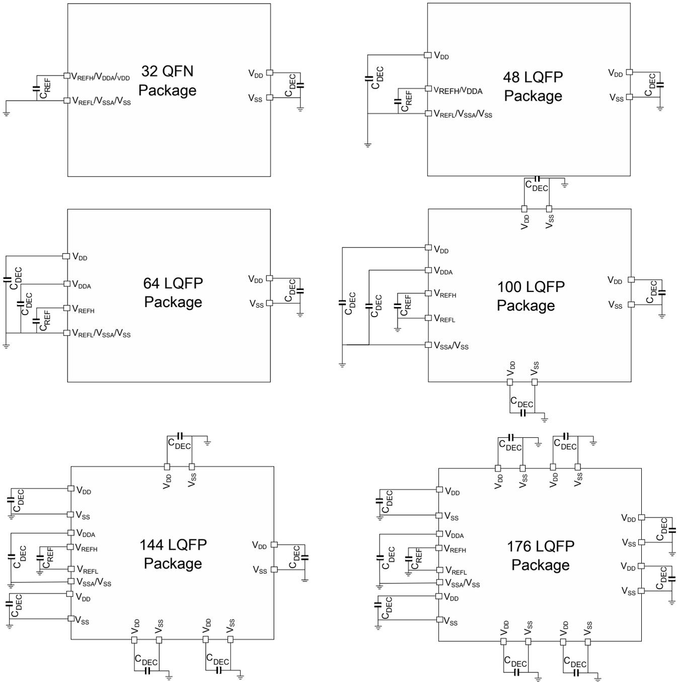
NOTE:  $V_{DD}$  and  $V_{DDA}$  must be shorted to a common source on PCB
