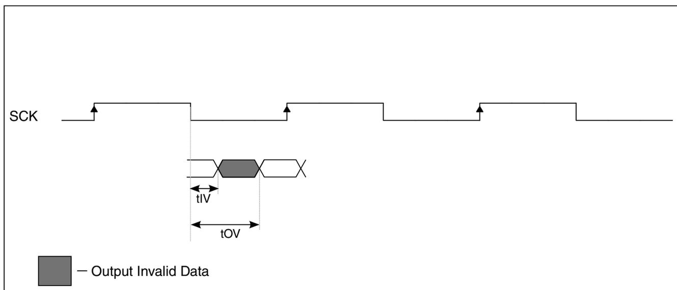
Figure 12. QuadSPI output timing (HyperRAM mode) diagram
