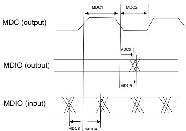
**Figure 28. MII/RMII serial management channel timing diagram**
