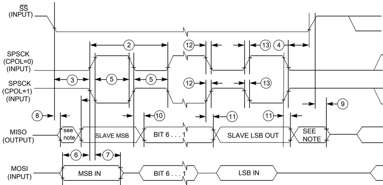
Figure 20. LPSPI slave mode timing (CPHA = 0)
