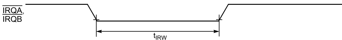
Figure 10-7 External Interrupt Timing (Negative Edge-Sensitive)
