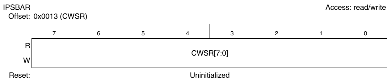
Figure 14-5. Core Watchdog Service Register (CWSR)
