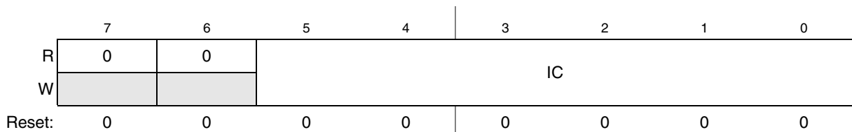
Figure 29-3. I 2 C Frequency Divider Register (I2FDR n )
