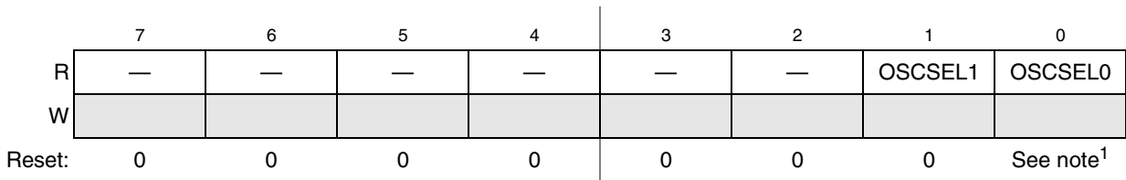
Figure 7-7. Clock Control Low Register (CCLR)
