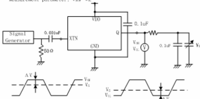
$V_s$  adjusted such that  $\Delta V=50 \times I_{\text{sr}}$
