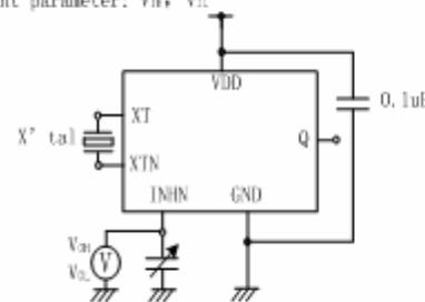
$V_{\text{dc}}$ : Voltage is 0V to  $V_{\text{dd}}$  transition that changes the output state.
