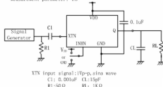
XTN input signal: 1Vp-p, sine wave
