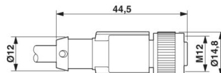
M12 x 1 socket, straight, shielded
