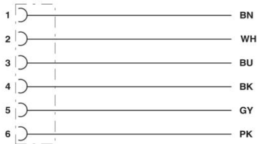
Contact assignment of M8 socket
