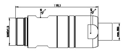
Shielded cable connector, long version M 40, cable entry 14-20.5 mm PE connecting earth pin to the shell 8 position male (4+3+PE)
