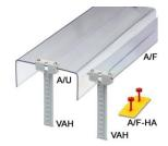
Flat-ribbon cover, for covering terminal strips, 2 mm thick, 9 cm wide, an additional requirement are 2 E/UK end brackets and 2 adjustable VAH cover holders. The max. supply length is 100 cm
