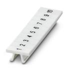
Zack marker strip, Strip, white, labeled, printed horizontally: consecutive numbers 1 ... 10, 11 ... 20, etc. up to 91 ... 100, mounting type: snapped, for terminal block width: 4.2 mm, lettering field size: 4.2 x 10.5 mm, Number of individual labels: 10
