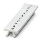
Zack marker strip, Strip, white, labeled, Printed vertically: consecutive numbers 1 ... 10, 11 ... 20, etc. up to 91 ... 100, mounting type: snapped, for terminal block width: 4.2 mm, lettering field size: 4.2 x 10.5 mm, Number of individual labels: 10
