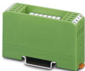
Indicator module, with 7 red LEDs and common return line, input voltage 24 V DC
