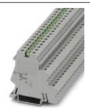
Sensor/actuator terminal block, connection method: Screw connection, cross section: 0.2 mm² - 4 mm², AWG: 24 - 12, width: 6.2 mm, color: gray, mounting type: NS 35/7,5, NS 35/15
