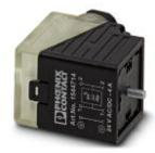
Valve connectors, 3-position, Valve connector A, connected with Z diode, Screw connection, cable gland M16, external cable diameter 5 mm  $\dots$  10 mm
