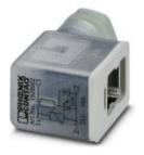
Valve connectors, 3-position, Valve connector B (10 mm), with 1 LED, connected with Varistor, Screw connection, cable gland Pg9, external cable diameter 6 mm ... 8 mm
