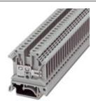
Feed-through terminal block, connection method: Screw connection, Slip-on connection, cross section:  $0.2 \text{ mm}^2$  -  $4 \text{ mm}^2$ , AWG: 24 - 12, width: 6.2 mm, color: gray, mounting: NS 35/7,5, NS 35/15, NS 32
