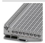
Potential distributors, nom. voltage: 500 V, nominal current: 24 A, cross section: 0.14 mm² - 4 mm², AWG: 12 - 26, connection method: Spring-cage connection, number of connections: 2, width: 5.2 mm, length: 141 mm, color: gray, mounting: NS 35/7,5, NS 35/15
