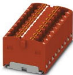
Distribution block, bridged internally, nom. voltage: 450 V, nominal current: 17.5 A, connection method: Push-in connection, number of connections: 18, cross section: 0.14 mm<sup>2</sup> - 2.5 mm<sup>2</sup>, AWG: 26 - 14, width: 37.4 mm, height: 17.7 mm, color: red, mounting type: for snapping onto a DIN rail adapter
