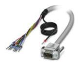
Assembled shielded round cable; connection 1: Single wires (9-position) (The wires are marked and fitted with ferrules. The braided shield is routed to a separate cable end.); connection 2: D-SUB pin strip (1x 9-position); cable length: 2 m
